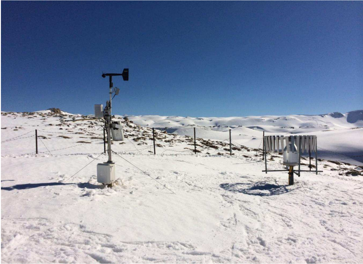
Fig. 3.3. Automatic weather station at Mzar (MZA) (2296 m a.s.l.) where all sensors are located on the tower and the precipitation gauge is located to the right of the station. Image captured on March 5th, 2015 (courtesy of the author).
