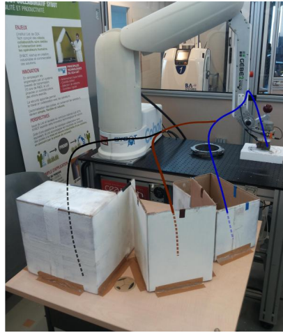
Figure 6.1: Multiple Virtual Guides created in the robot workspace for the Pick-and-Place Experiment presented in [Raiola 2017a]. The task consisted in taking 6 discs from the robot's workstation and insert them inside specific boxes identified with 3 different colors: blue, brown and black. For each box there were two discs with a piece of tape of the same color.
