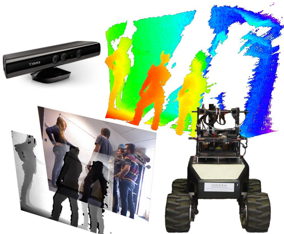
(c) Embedded Kinect camera on a Robotnik Summit XL robot that allows to obtain low cost RGBD images. Image inspired from [Guerry 2017], where new neural networks fusion approaches using RGBD images are applied for people detection tasks in robotic exploration.
