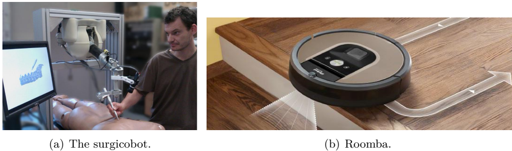
Figure 1.4: Examples of recent innovative human-robot interfaces and sensors. a) The Surgicobot robot. Designed for milling assistance, especially in orthopedic surgery. It was developed by HAPTION (Laval, France) as part of the Surgicobot project (ANR Tecsan). Image extracted from [François 2013a], where different control strategies for Surgicobot are proposed. b) iRobot Roomba Vacuum service robot. This mobile robot is equipped with a camera that allows it to navigate using VSLAM (Vision Simultaneous Localization and Mapping).
