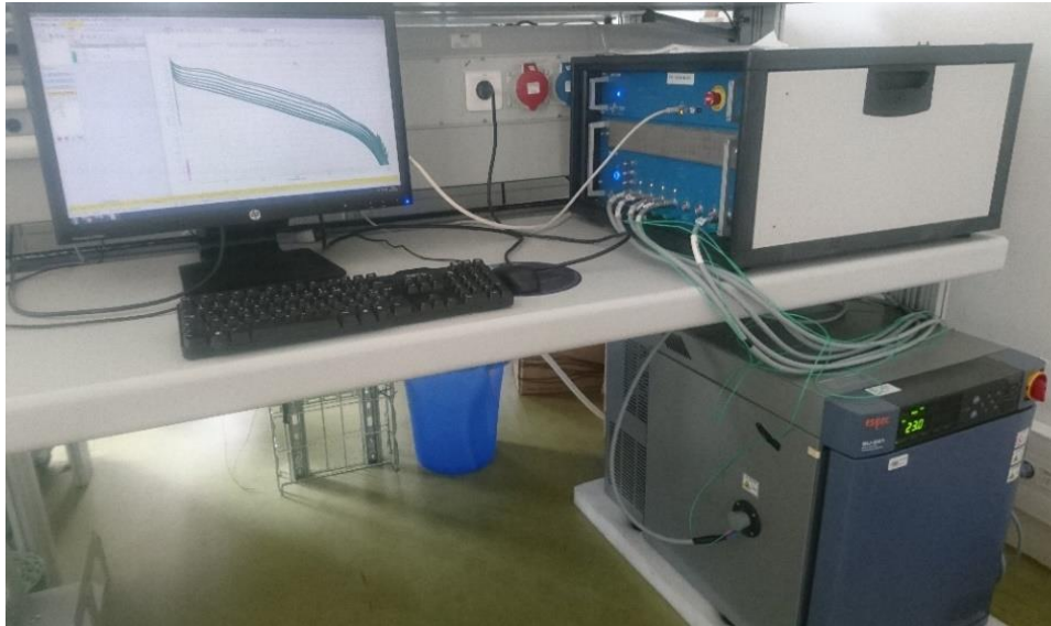
Figure 3.22 Experimental setup for cycling batteries
