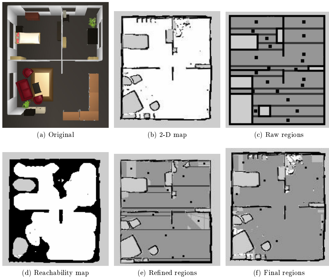
Figure 6.2: View point selection process. The boundaries of the 2-D map are extended, horizontally in this case. Small and unreachable regions are removed. Regions with similar view points are merged.
