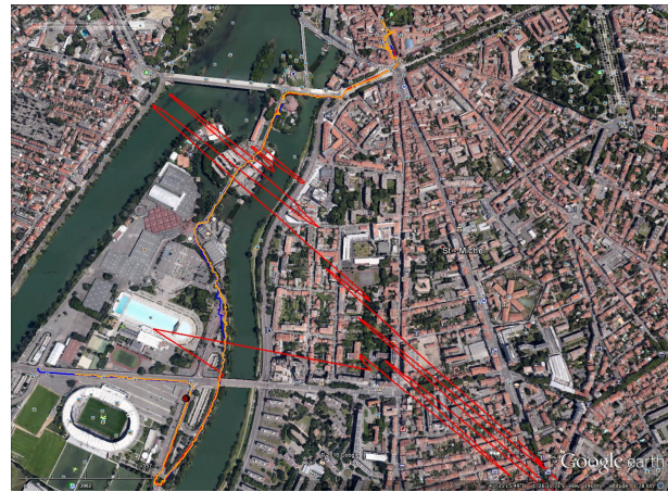
Fig. 3. Position given by a noiseless GPS receiver X(t) (color orange), by a faulty GPS receiver without adding the fault tolerant technique (color red), by a faulty GPS receiver when using the fault tolerant technique (color blue), displayed using Google earth
