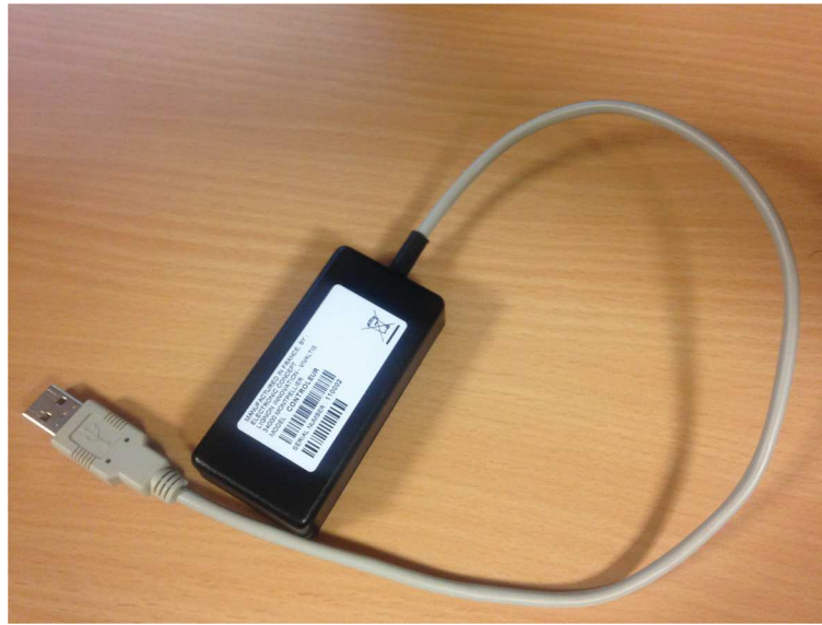
Fig. 3 The communication/control unit of the wireless stimulator
