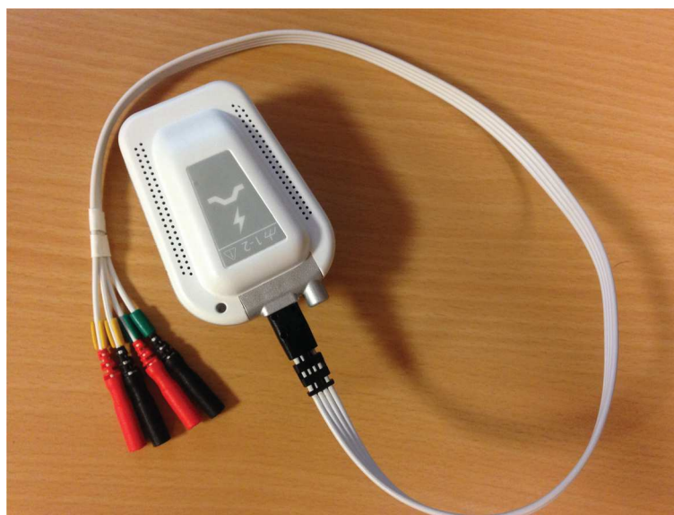
Fig. 2 The wireless stimulator is a regulated-current dual-channel stimulator with the features as follows. Maximal electrical current is 100 mA, stimulation frequency ranges between 1 to 1000 Hz, and electrical polarity can be configured. All parameters are dynamically and remotely adjustable
