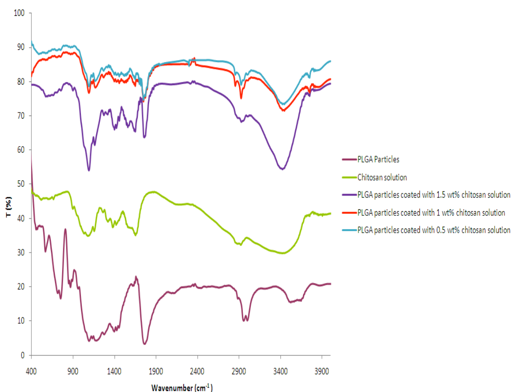
Figure 5.13 FTIR spectroscopy of uncoated PLGA particles, chitosan solution and PLGA particles coated with chitosan solution of three different concentrations.
