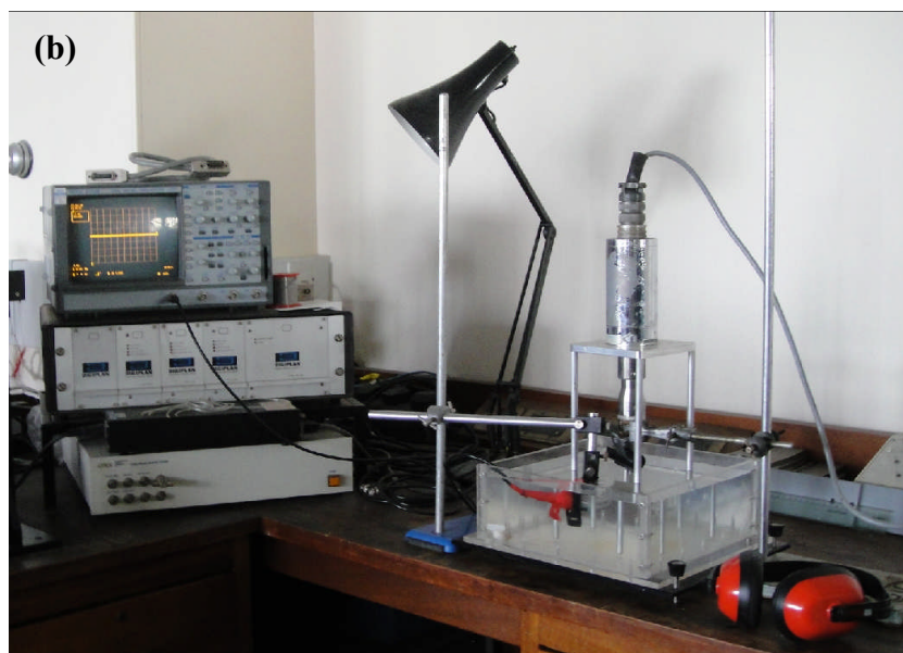
Figure 3.5 (a) Schematic and (b) real apparatus used for ultrasound exposure and acoustic emission measurements.
