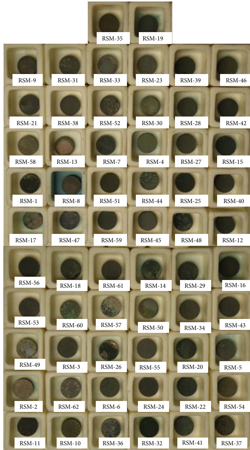
FIGURE 2: Pictures of Ni-(0~15)Co-(8~15)Cr-(0~5)Mo-(0~10)W-(3~8)Al-(0~5)Ti-(0~10)Ta-0.1C-0.01B alloys after oxidation tests at 850°C.
