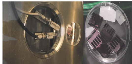
FIGURE 4: Organic cells used for testing.
