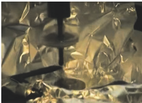
FIGURE 2: 40 nm PDOT:PSS coating (1 min spin coating at 3000 rpm).
