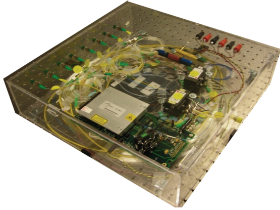
FIGURE 4: Picture of the beamformer based on a dispersive prism.
