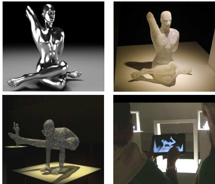
Figure 28: Virtual model of Yoga Asana – Gaumukhasana (top left), Rapid Prototype manufactured sculpture (top right), 3D animation of virtual gallery (bottom left), Augmented Reality experience on tablet (bottom right)
