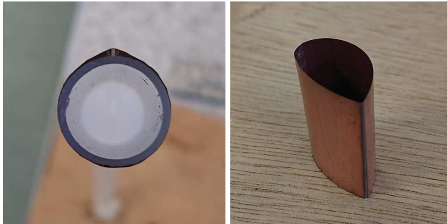
(a) Top-down view showing bending around the slot. (b) Sensor off-pipe showing Mylar bending.
