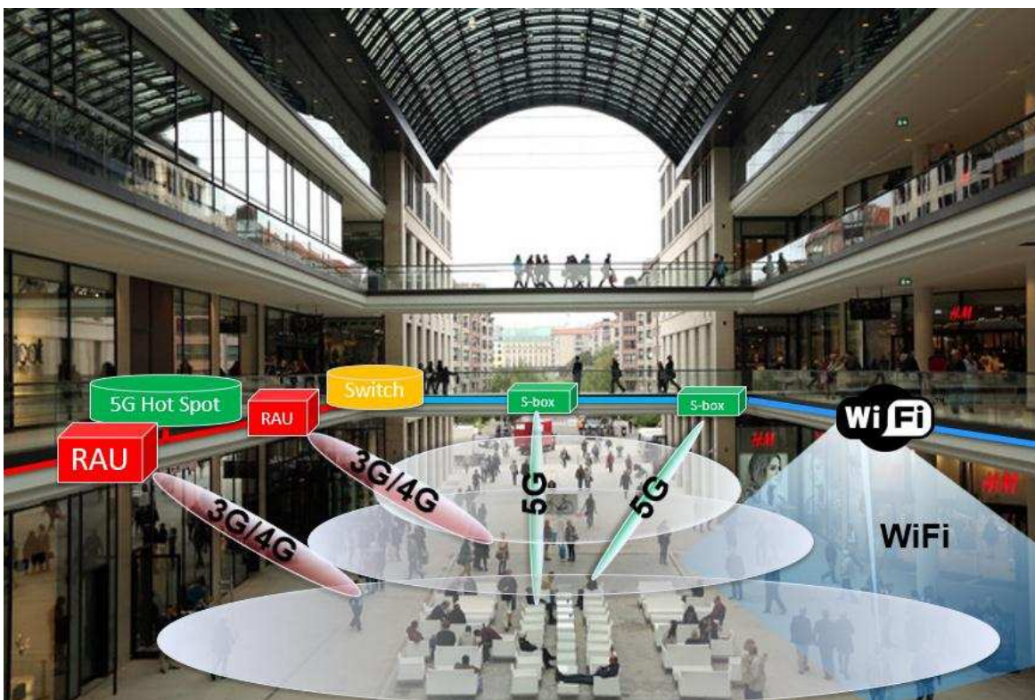
Figure 1: Illustration of the shopping mall field trial for demonstrating switchover in a heterogeneous network (WiFi & 60 GHz) and a 60 GHz hot spot
