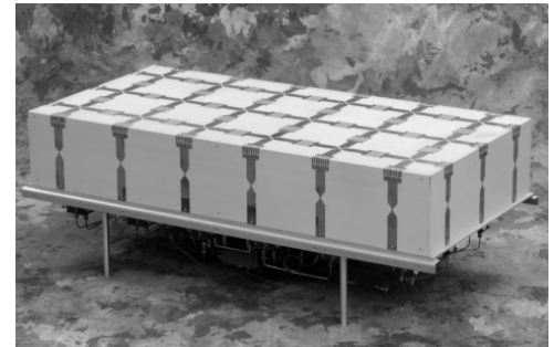
FIGURE 7. TCDA breadboard for VHF/UHF band [4]
