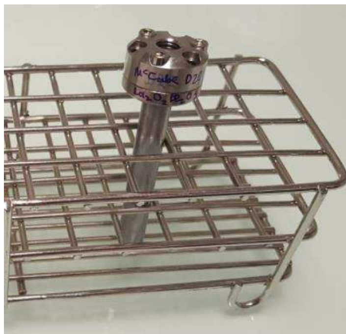
Figure 2.08 Sample in vanadium can ready for neutron diffraction measurements
