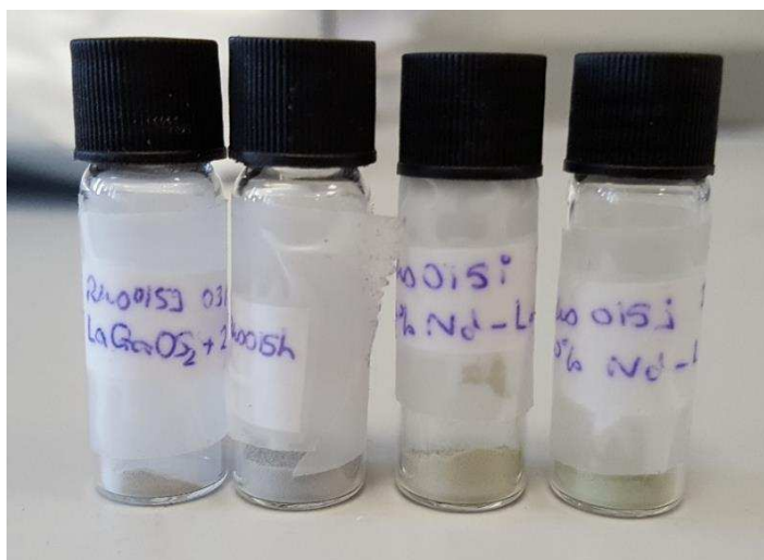
Figure 5.08 Colour change in each of the different Nd doping concentrations from the initial blue-green colour after reaction. \text{La}_{0.98}\text{Nd}_{0.02}\text{GaOS}_2 (far left) became pale-grey, \text{La}_{0.95}\text{Nd}_{0.05}\text{GaOS}_2 (second from the left) became pale-grey, \text{La}_{0.93}\text{Nd}_{0.07}\text{GaOS}_2 (third from the left) became green-grey and \text{La}_{0.9}\text{Nd}_{0.1}\text{GaOS}_2 (far right) became apple-green.
