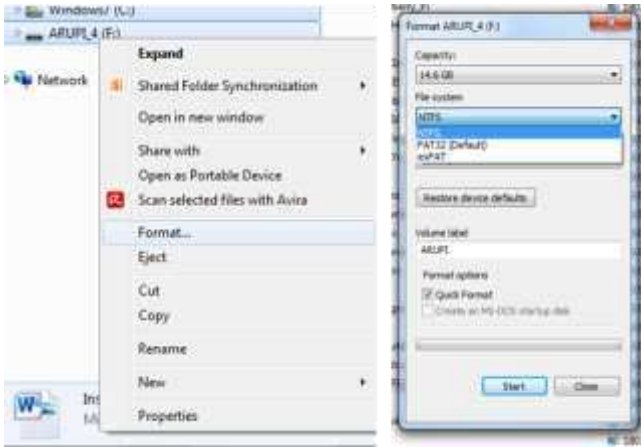
Figure 2. Format USB drive to NTFS file format – right click on the USB drive in Windows explorer; select <Format>; File System = <NTFS>; <Start>. This step is important.
