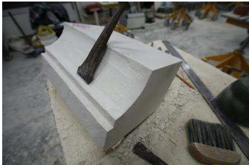
[Figure 4-18 A claw chisel removing excess stone after the punch tool was used. Photo by the author.]
