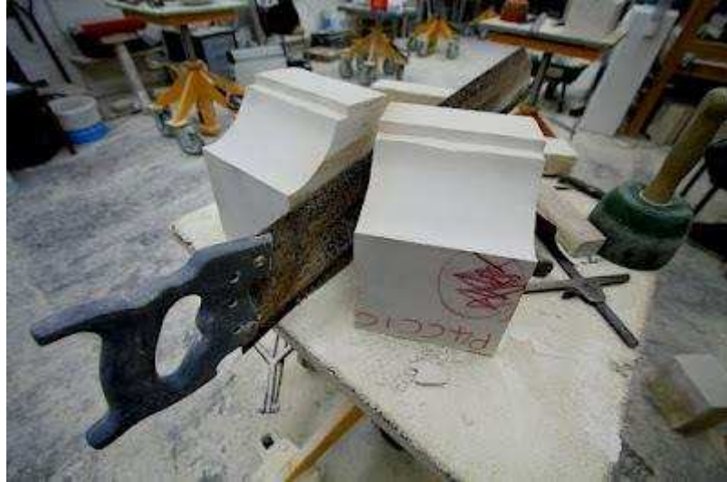
[Figure 4-19 A tungsten saw blade used to cut the stone. Photo by the author.]
