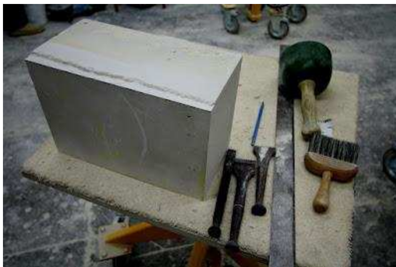
[Figure 4-6 The marginal draft created by the drafting chisel. Photo by the author.]
