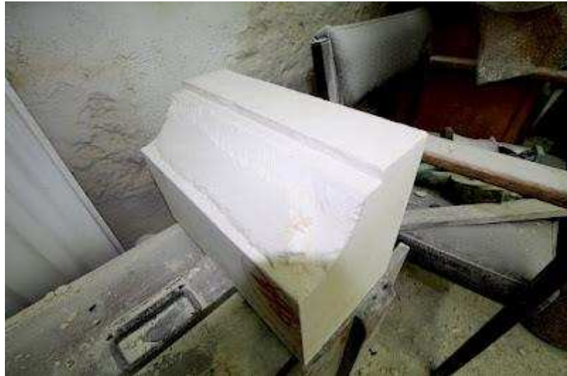
[Figure 4-17 The curved moulding profile with marginal drafts defining the edge of the moulding curve. Photo by the author.]
