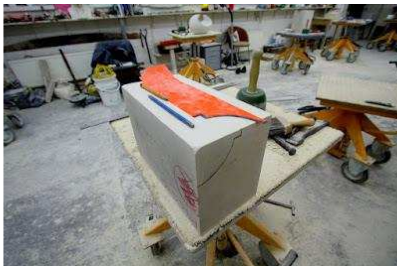
[Figure 4-13 A scribe and acrylic template sit atop the stone with profile inscribed. Photo by the author.]
