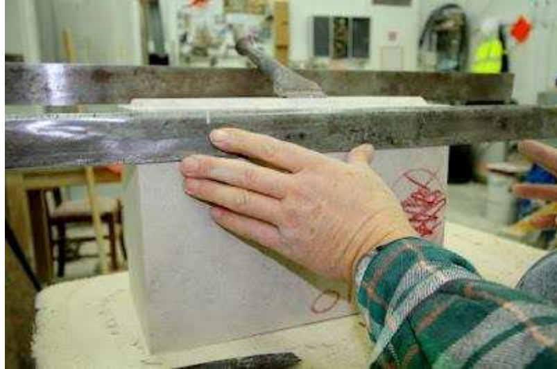
[Figure 4-9 Sighting through the marginal drafts with straight edges held in place by a chisel. Photo by the author.]
