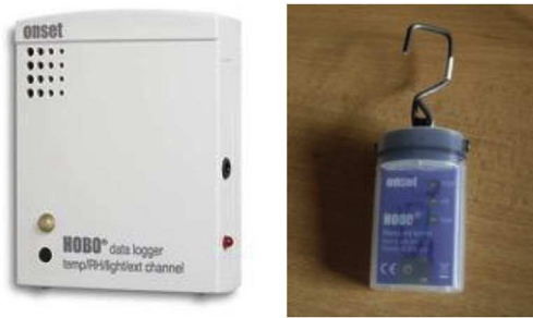
Fig. 5. Indoor temperature sensors (Hobo U-12 [Left], Hobo Pendant [Right]) [48].
