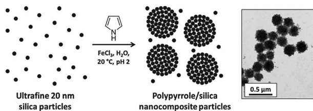
Fig. 6 Schematic representation of the synthesis of polypyrrole/silica nanocomposite particles by oxidative polymerisation of pyrrole in the presence of an aqueous silica sol. A representative TEM image of polypyrrole/silica nanocomposite particles is shown on the right.
