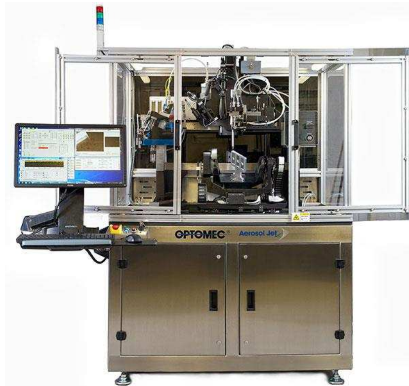
Figure 2-6 The aerosol printer from Optomec [8]
