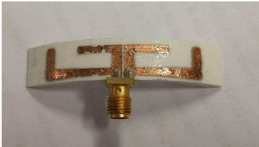
Figure 7-9 Optomec printed antenna on an FDM printed bracelet
