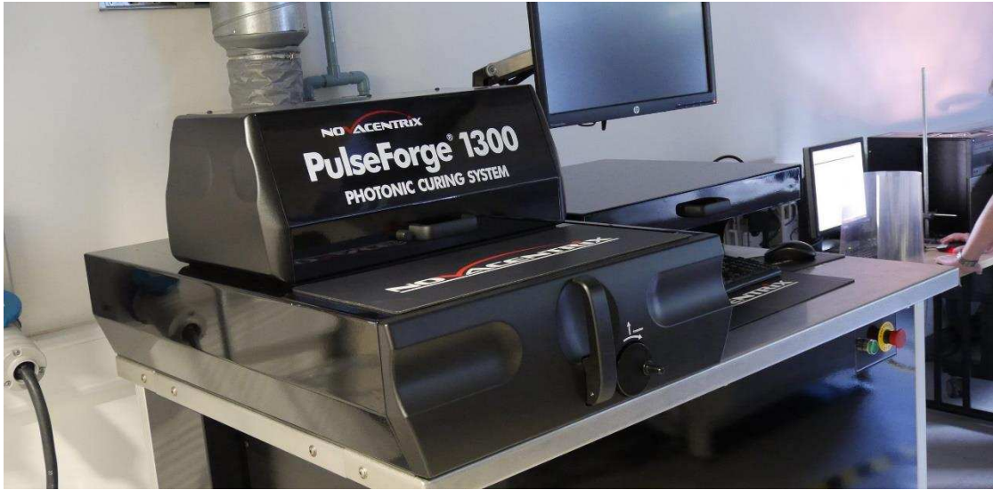
Figure 2-8 PulseForge machine from Novacentrix [10]
