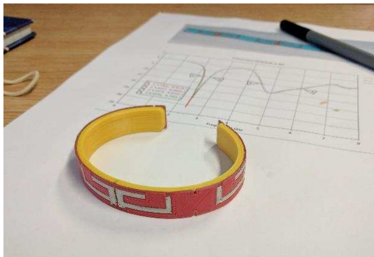
Figure 7-8 Printed bracelet antenna
