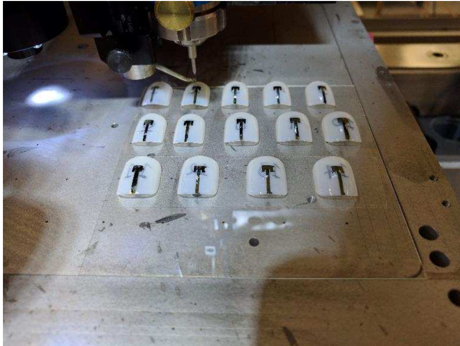
Figure 8-7 Printed antennas using the Optomec machine
