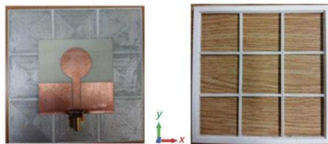
Figure 2-13 3D printed EBG configuration and stencil [51]
