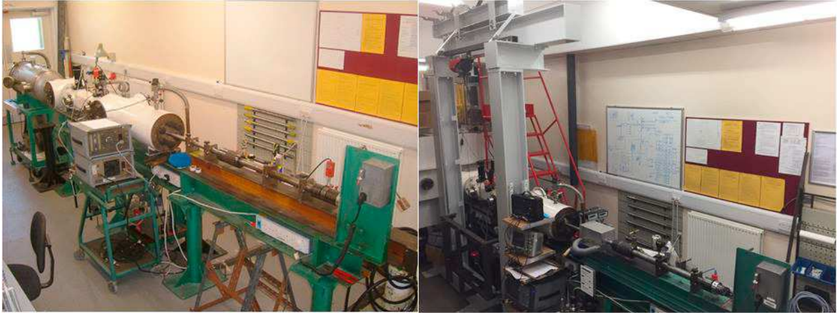
Fig. 1. The light gas gun at the University of Kent (circa 2008). The left image shows the gun before any major modifications. The right image shows the gun as of April 2017 with the most obvious addition being the grey framework that is the support structure for the vertical firing axis.
