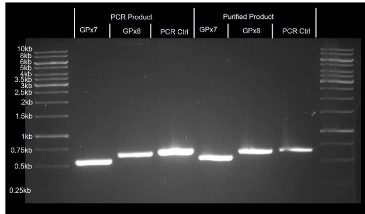
Fig 3.15. Native GPX7 and GPX8 PCR generated DNA products and purified PCR generated DNA products. Following the unsuccessful previous attempt PCR was repeated with three fold as much PCR generated DNA product (wells 2-4) and purified PCR generated DNA products (wells 5-7) of GPX7 (wells 2 and 5), GPX8 (wells 3 and 6) and a PCR control of a reaction shown previously to work (GPX8 for pBEVY-L) (wells 4 and 7).
