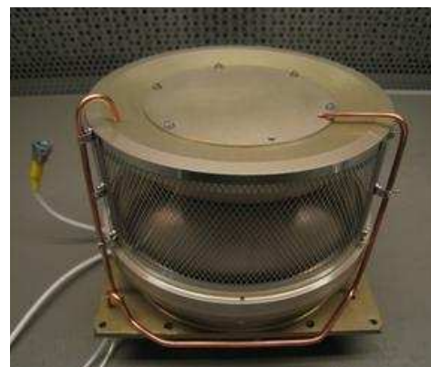
The Electron Analyser System for the Solar Wind Analyser on Solar Orbiter, currently being built at MSSL. Image credit: MSSL.
