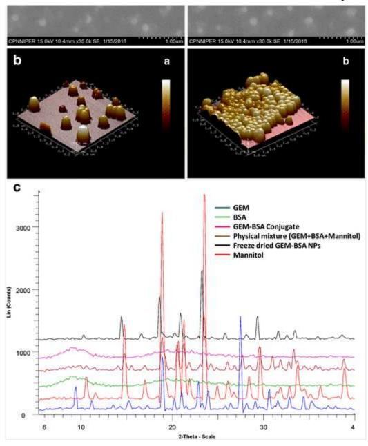
Powder X-ray diffraction analysis (PXRD)
