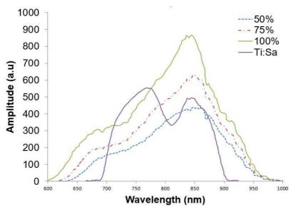
Fig.1. Spectrum at the output of the two sources: SC running at different output power (50%, 75% and 100%) and Ti:Sa laser.
