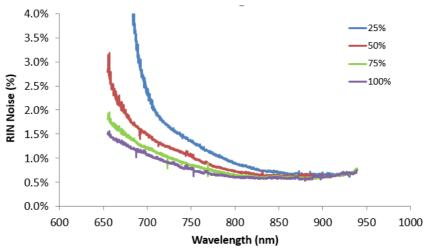
Fig.3. Relative Intensity Noise (RIN) versus wavelength for different output power levels of the SuperK.
