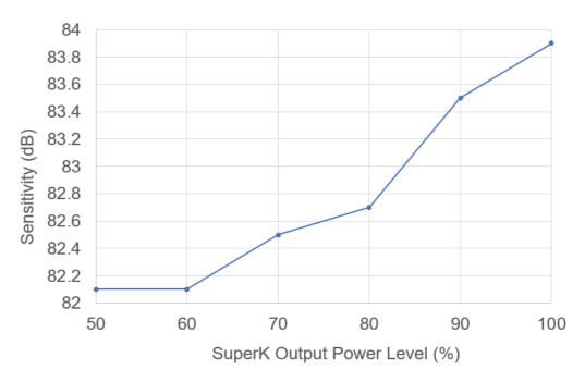
Fig.2 Sensitivity as a function of the percentage output from the SuperK. The power on the sample was  $400\mu W$ .
