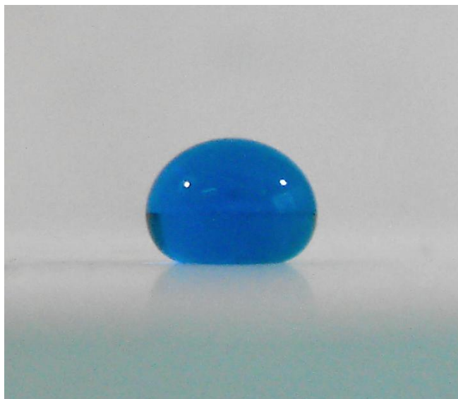
Figure 5.06. Photograph showing a 10 \mu\text{L} water droplet on microscope slide coated with Sylgard 184 via dip-coating then AACVD.
