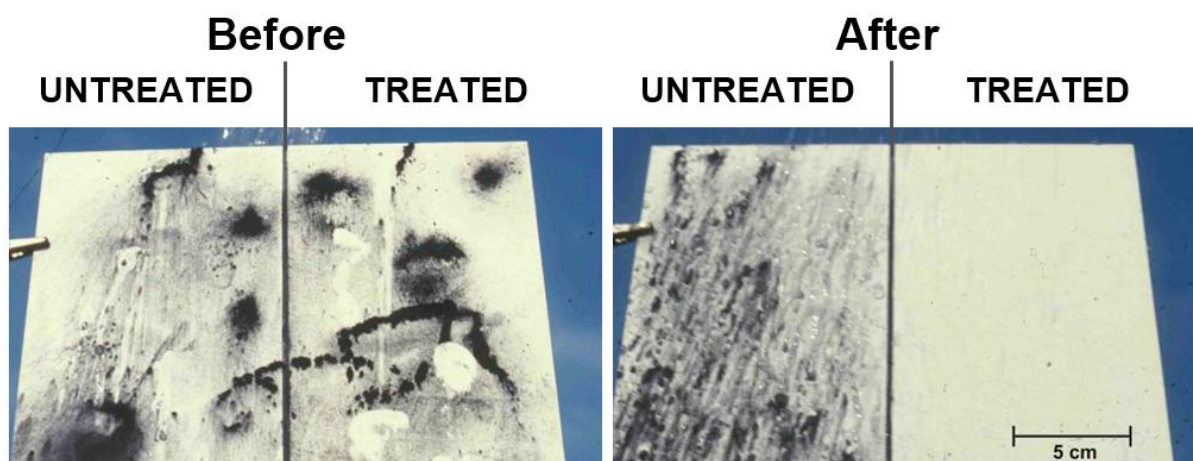
Figure 1.42. Soot-coated Formica plates. The side of the left plate is untreated and shows no Lotus-effect self-cleaning and soot removal with action of water is inefficient. The right side of the plate is coated with micropowdered PTFE giving the surface superhydrophobic properties, from which soot is easily removed with water. 132
