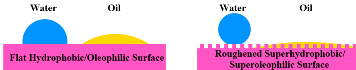
Figure 7.02. Schematic showing the interaction of water and oil with hydrophobic/oleophilic surfaces upon roughening.
