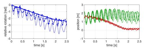
Figure 5.9: Motion of the free joint and the tip node of the generic manipulator. Blue: joint; red: x; green: y. Dotted: rigid joints; Dashdotted: adding of spring elements; Solid: adding of spring and damper elements.
