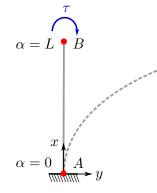
Figure 3.1: Continuum arm subject to a torque  $\tau$  at its free end. Solid line: initial configuration. Dashed line: deformed configuration.
