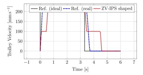
Figure 6.32: Velocity commands for the ZV-IPS experiments.
