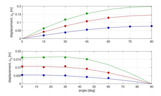
Figure 6.10: Tip displacements of the Princeton cantilevered arm subjected to the end load P with three different intensities and seven configurations. Blue:  $P_1$ , red:  $P_2$ , green:  $P_3$ . Scatter: experimental data, dotted: numerical predictions from SimSOFT.
