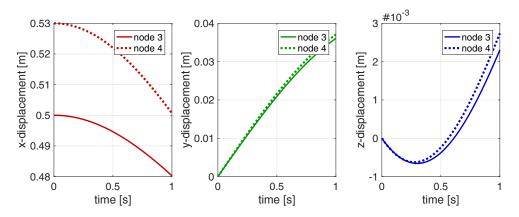
Figure 6.22: Displacements of the Magellan Robotic Catheter 10Fr in the test simulation. As we can see, the trajectory induces a three-dimensional out-of-plane motion.
