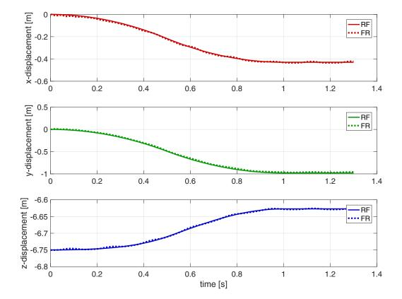
Figure 6.17: Displacements of end-effector of the hybrid kinematic mechanism in the test trajectory.
