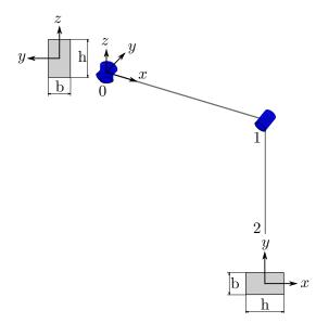
Figure 6.5: The spatial flexible manipulator, constituted by two links with two active joints, one universal, one revolute.
