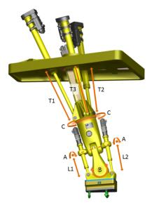
Figure 6.14: Hybrid kinematic mechanism for DEMO MMS remote handling
