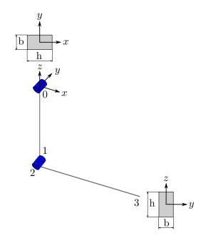
Figure 6.3: Flexible double pendulum in its initial configuration.
