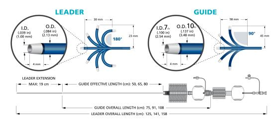
Figure 6.19: Geometric data for the Magellan Robotic Catheter 10Fr
