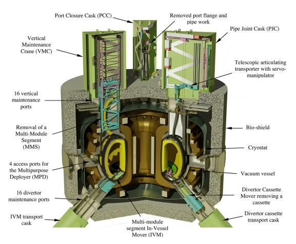
Figure 6.13: A qualitative picture of the DEMO vertical maintenance system architecture.
