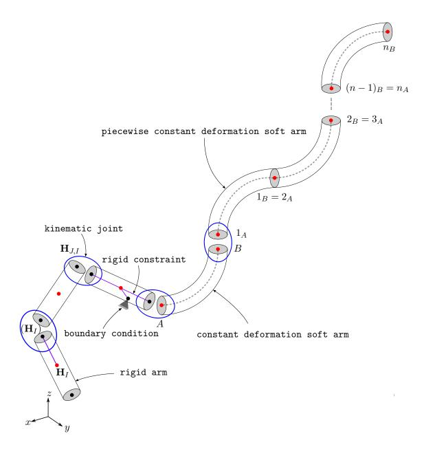
Figure 5.3: A generic robotic mechanism.  $\mathbf{H}_{I}$  are nodal frames,  $\mathbf{H}_{J,I}$  are relative frames and  $(\mathbf{H}_{I})$  are optional frames.
