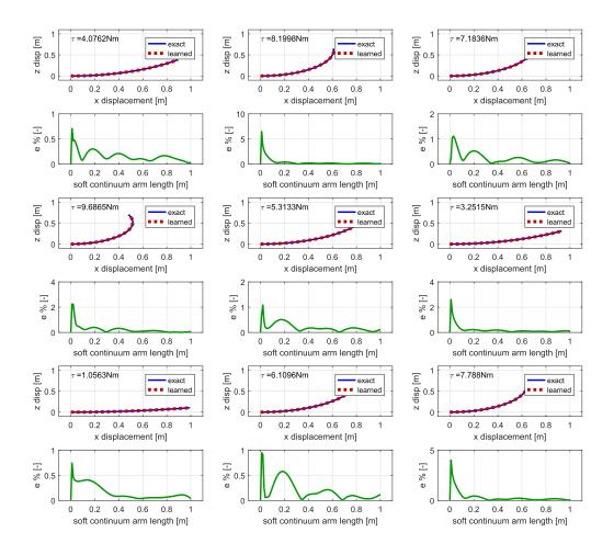
Figure 6.26: Learned continuum arm model at different load conditions.
