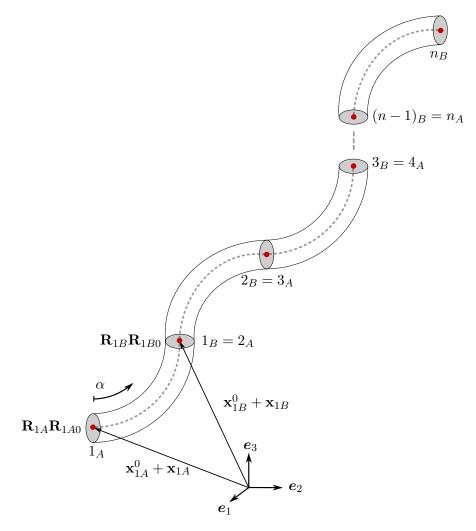
Figure 2.2: Kinematics of the piecewise constant deformation model
