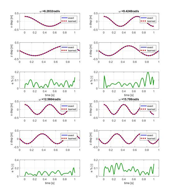
Figure 6.27 shows the errors of the learned model in four different configurations. In all these cases, the average errors are below 1%.
