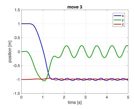
Figure 6.8: Tip displacements of the spatial flexible manipulator for move 3
