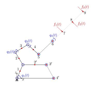
Figure 5.8: Schematic model of a generic robotic mechanism composed by rigid and soft arms structured in a parallel and serial topology.
