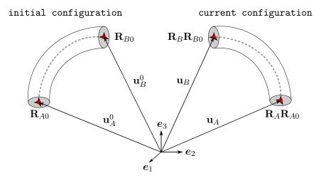
Figure 2.3: Constant deformation soft arm in its initial and current configuration.
