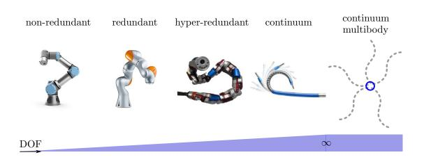
Figure 1: Classification of robots based on degrees of freedom. (Images: from left, © 2017 Universal Robots A/S; © 2017 Kuka Robotics Corp.; Choset's Modsnake; © 2017 Hansen Medical Inc.)
