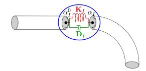
Figure 5.2: Schematic representation of a revolute elastic joint.
