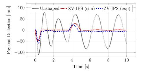
Figure 6.33: ZV-IPS: comparison of experimental and simulated response.
