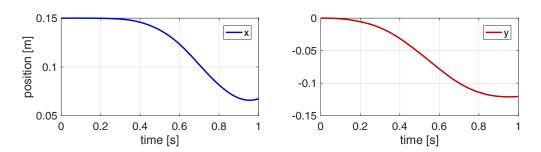
Figure 6.25: Tip displacements of the soft bending actuators along the test trajectory  $% \left[ {{{\mathbf{x}}_{i}} \right]_{i = 1}^{i - 1}} \right]$
