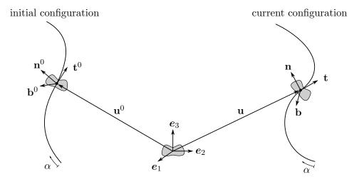
Figure 2.1: Geometric description of the reference curve for the continuum arm.
