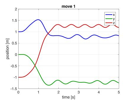
Figure 6.6: Tip displacements of the spatial flexible manipulator for move 1
