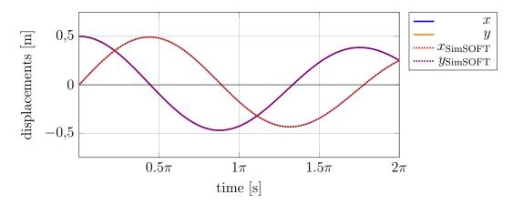
Figure 6.2: Displacements of the tip-position of the two-link rigid manipulator in the inertial reference frame.
