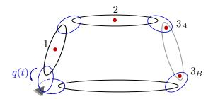
Figure 5.6: A four-bar mechanism.
