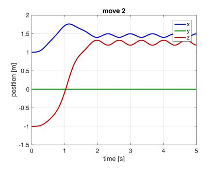
Figure 6.7: Tip displacements of the spatial flexible manipulator for move 2
