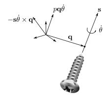
Figure 1.2: A screw axis S represented by a point  $\mathbf{q}$ , a unit direction vector  $\mathbf{s}$  and a pitch p.
