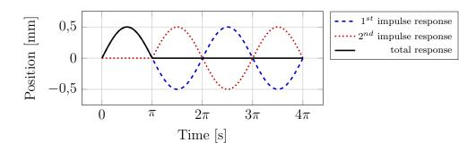
Figure 6.28: Zero vibration input shaping process
