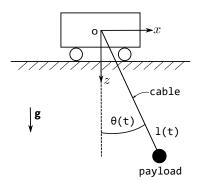
Figure 6.30: Nonlinear pendulum.
