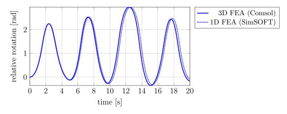
Figure 6.4: Relative angular position of the revolute joint for the flexible double pendulum. Solid: 1D FEM, dashdotted: 3D FEM
