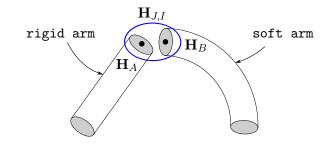
Figure 5.1: A kinematic joint which connects two generic arms of a robotic manipulator.
