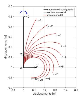
Figure 3.2: Cantilevered soft arm subject to a torque  $\tau$  at its free end. The initial configuration is a straight vertical line, while the deformed configuration is a planar curve of constant curvature.
