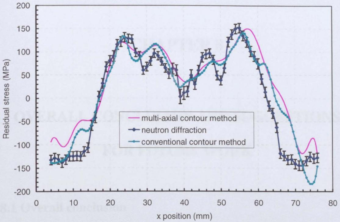
Figure 7.7 Longitudinal residual stress at the  $\theta = 0^\circ$  surface along the line  $y = 3.55$  mm.
