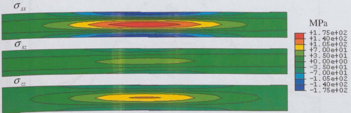
Figure 6.12 Non-zero components of residual stress variation on the  $\theta = 0^\circ$  surface for 3D numerical validation of the multi-axial contour method.
