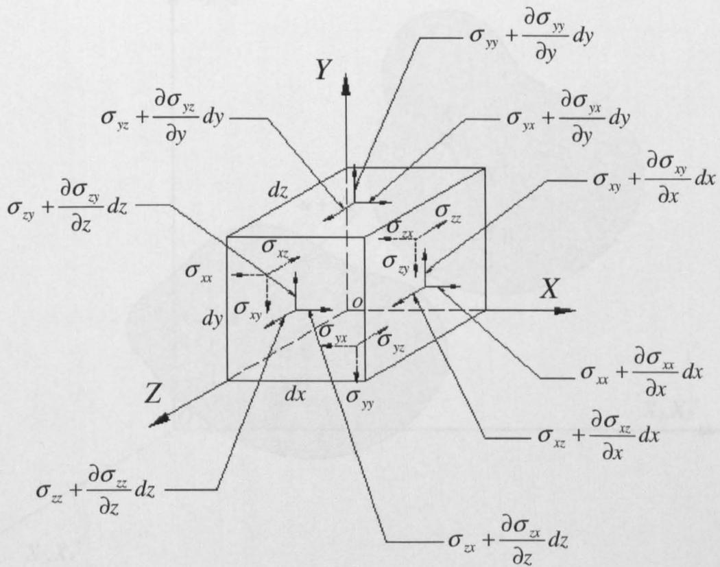
Figure 2.5 Equilibrium stress components on infinitesimal cubic elements.
