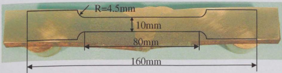
Figure 4.7 The dimensions of the standard tensile test specimen and its machining position on the slice taken from the girth weld.
