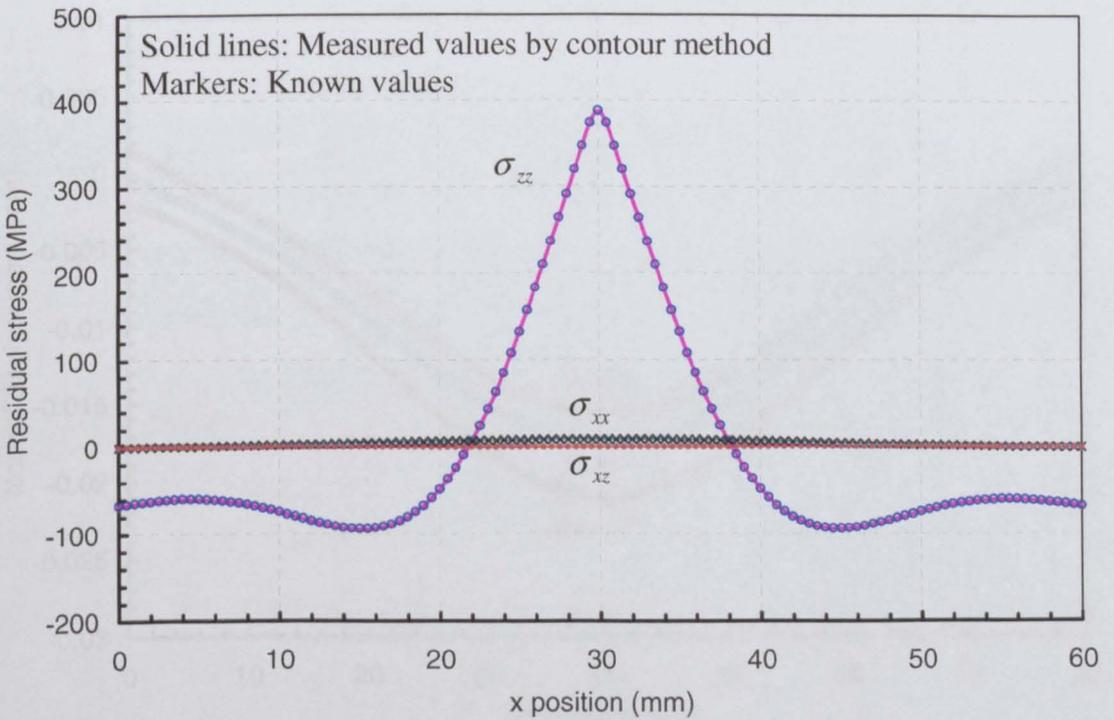
Figure 6.8 Residual stress results for 2D multi-axial contour simulation.
