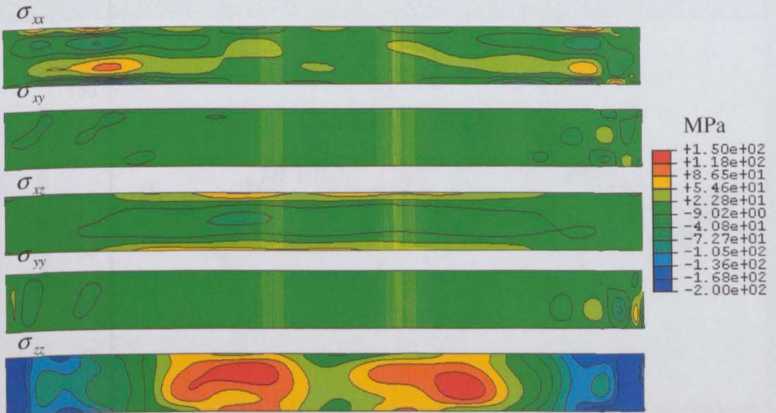
Figure 7.6 Non-zero components of residual stress variation on the  $\theta = 0^\circ$  surface for VPPA welded sample.
