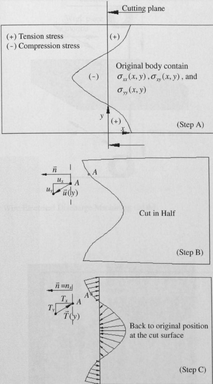
Figure 5.1 Illustration of Bueckner's superposition principle. Point A symbolizes any arbitrary point on the cut plane with its displacement and surface traction components.
