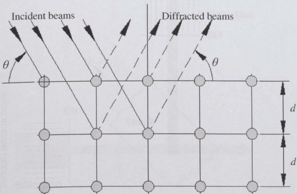
Figure 2.13 Bragg's Law - Diffraction of X-rays by a crystal.
