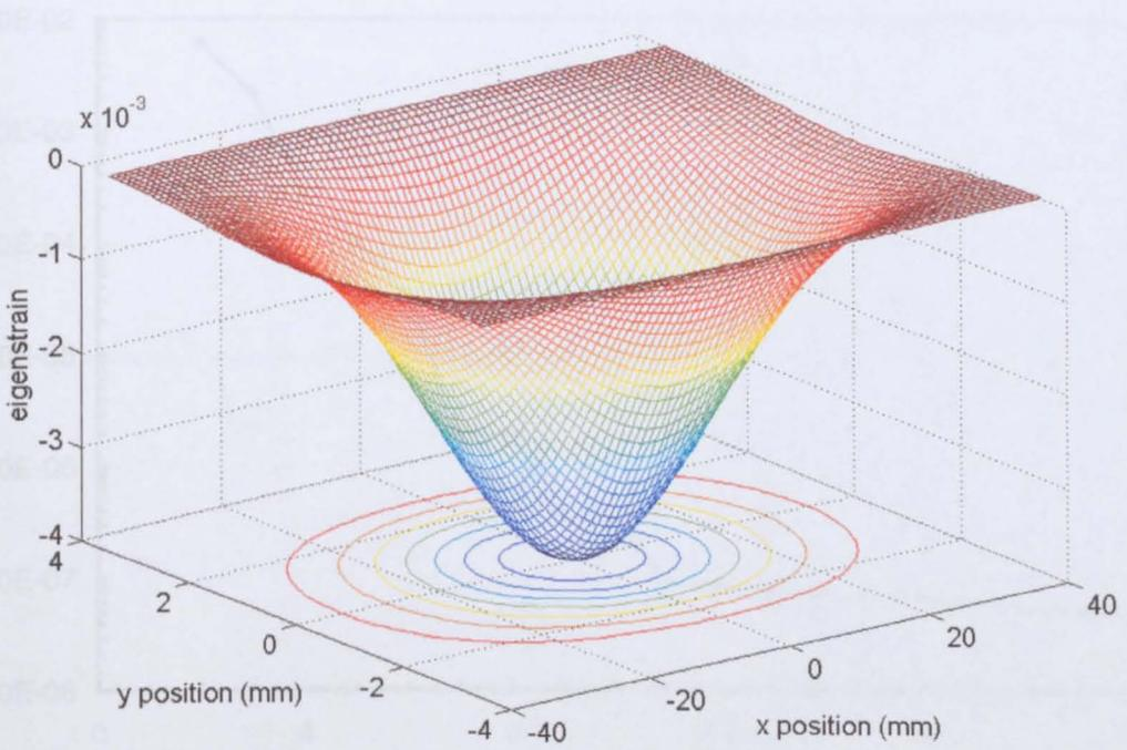
Figure 6.5 Eigenstrain distribution on the cross-sectional area for the numerical validation of the multi axial contour method
