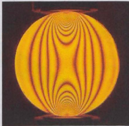
Figure 3.2 Isochromatic fringes in a disc of uniform thickness compressed across its vertical diameter [3].
