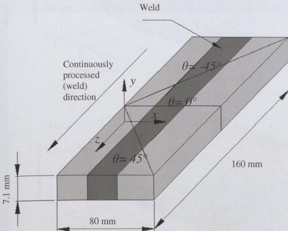
Figure 7.2 VPPA welded 2024-T351 aluminium alloy sample used for multi-axial contour method.
