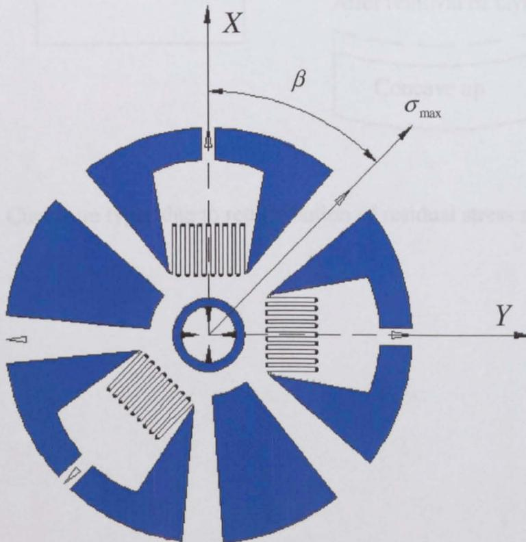
Figure 2.9 ASTM type hole drilling strain gauge rosette [22].
