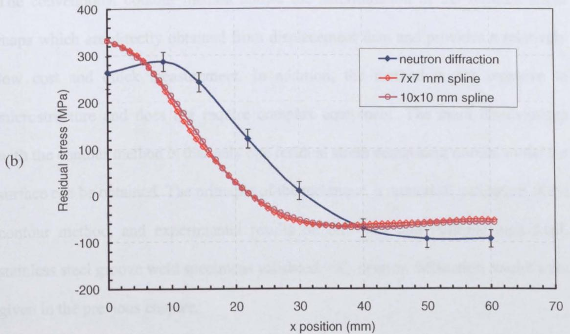
Figure 5.27 Comparison of the residual stresses determined by neutron diffraction and contour method results obtained from the (a) 3.5×3.5 mm, 5×5 mm splines (b) 7×7 mm, and 10×10 mm splines, along scan C of the 3 pass groove weld specimen.
