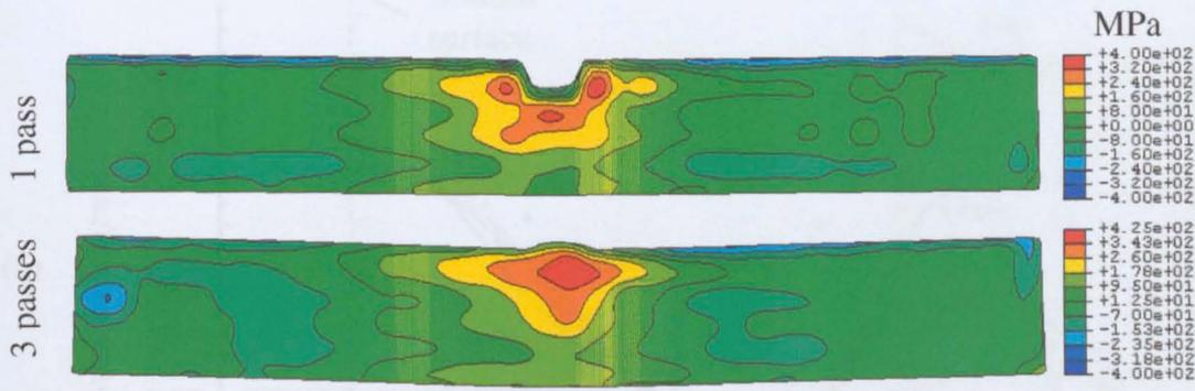
Figure 5.16 Preliminary contour results on the 1-pass and 3-pass groove weld specimens
