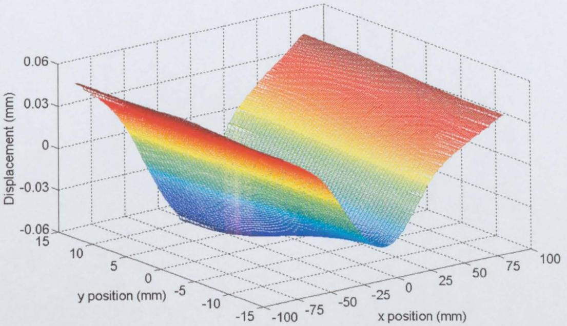
Figure 5.15 5×5 mm cubic spline function fitted to 1 and 3 pass averaged surface contour measurement.
