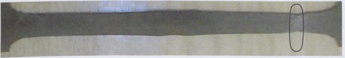
Figure 4.25 A photograph of the standard sample after tensile test. The marker shows the position of the sample where necking starts.
