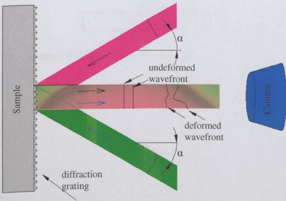
Figure 3.4 A schematic of the moiré interferometry system [5].
