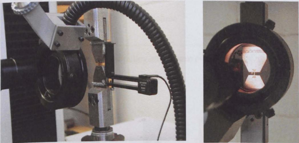
Figure 4.9 DIC set up for the full field strain measurement on the micro sample.
