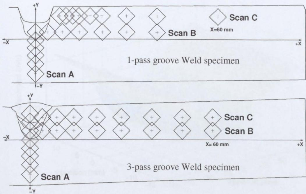
Figure 5.12 Schematic showing neutron diffraction measurement positions within each pass groove weld specimen, at the measurement plane.
