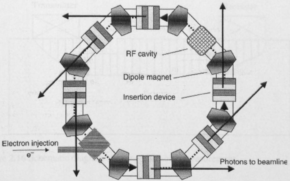
Figure 2.14: Schematic design of a storage ring [32].
