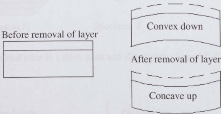
Figure 2.11 Curvature types due to redistribution of residual stress after removal of a layer.
