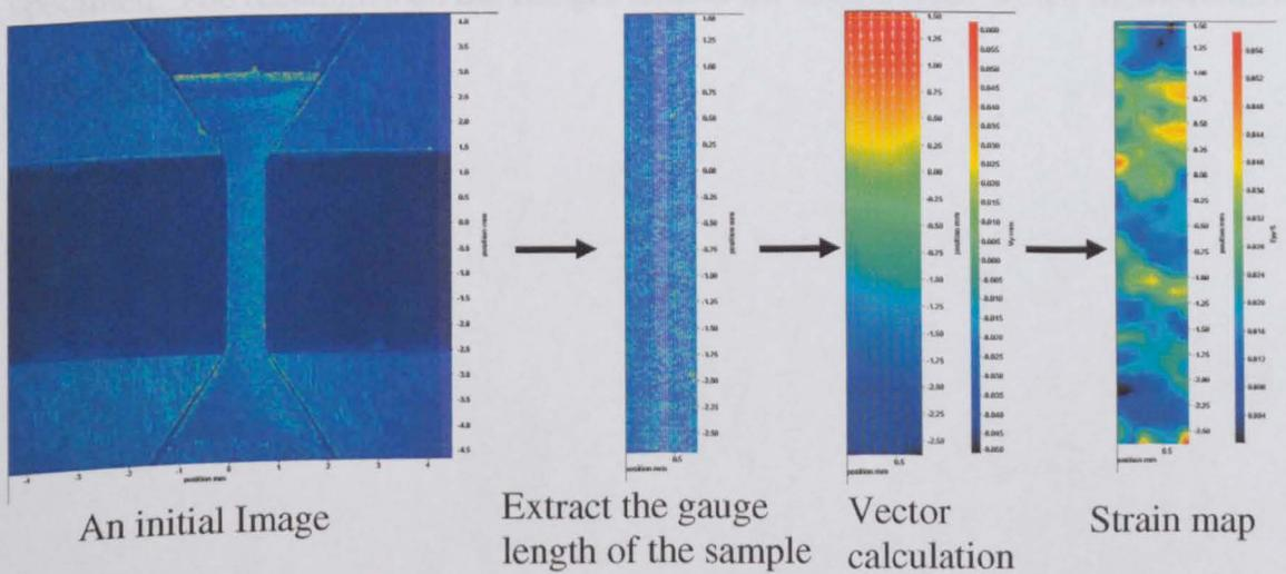
Figure 4.11 The post-processing steps of the analysis performed for one of the selected micro samples.
