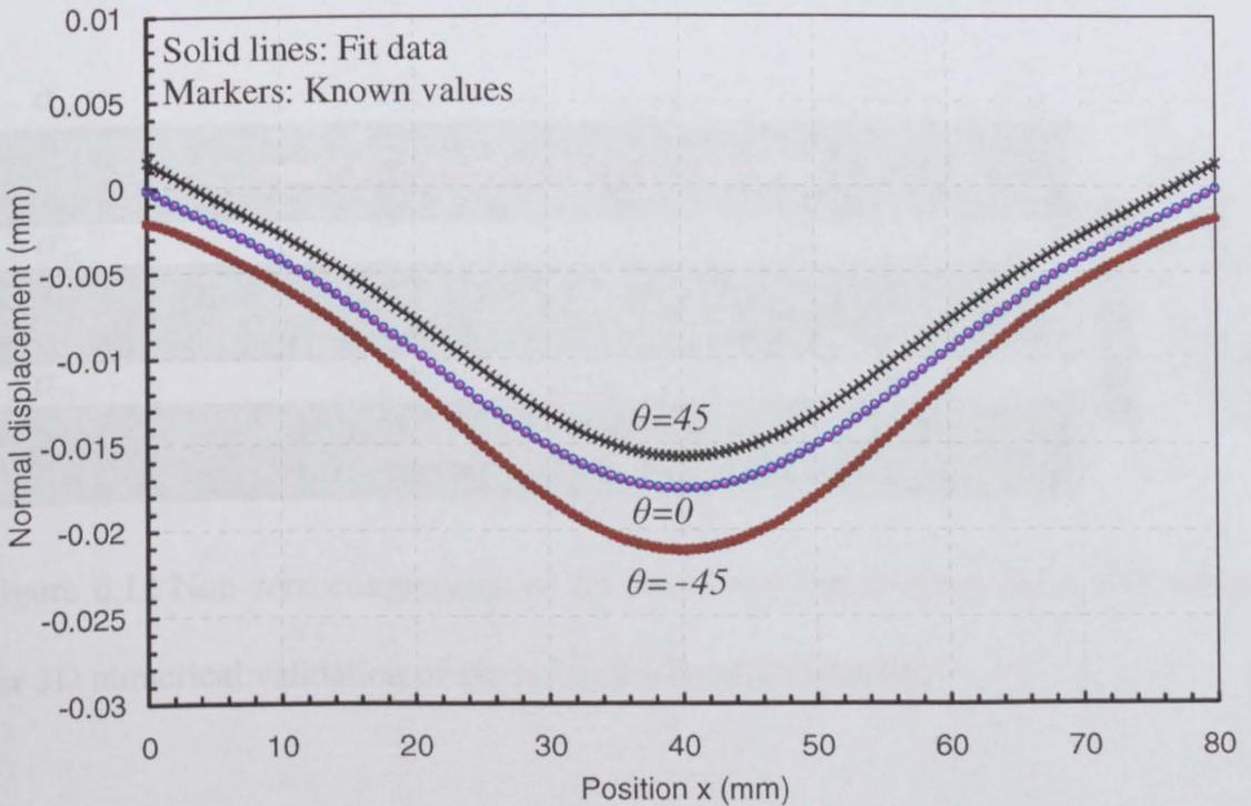
Figure 6.10 Comparison between known and fit data for 3D numerical verification of multi-axial method along the line  $y = 3.55$  mm.
