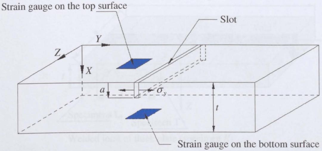
Figure 2.10 The crack compliance specimen geometry [23].
