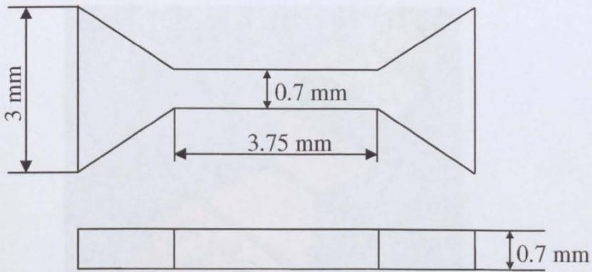
Figure 4.5 Schematic of a micro tensile test specimen
