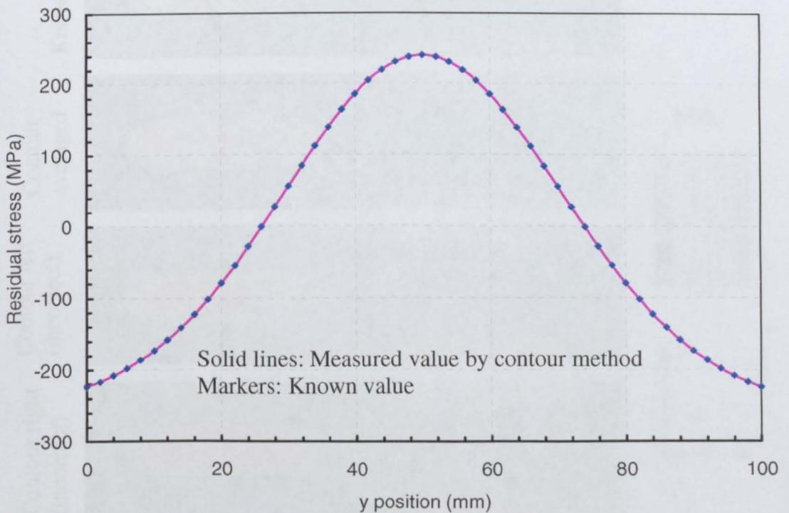
Figure 5.7 Comparison of known and measured residual stress for 2D numerical verification of contour method along the cut line
