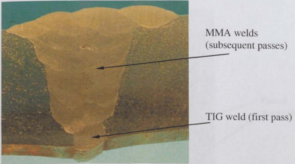
Figure 4.2 A macrograph showing the fusion boundary of weld and the positions of TIG and MMA welds.
