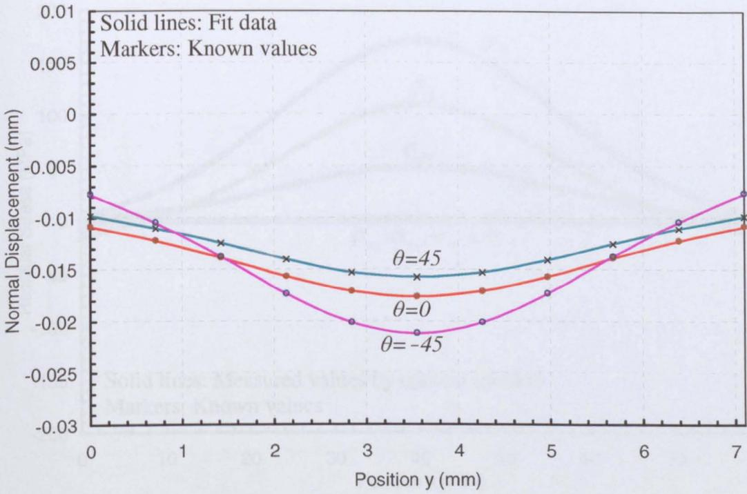
Figure 6.11 Comparison between known and fit data for 3D numerical verification of multi-axial method along the line  $x = 40$  mm.
