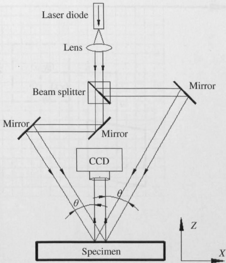
Figure 3.5 A schematic diagram of the ESPI system [13].
