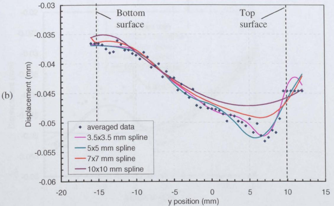
Figure 5.17 The comparison between the averaged data and four different spline knot spacings for the 1-pass groove weld specimen along the lines (a)  $x=0$  mm and (b)  $x=8$  mm.
