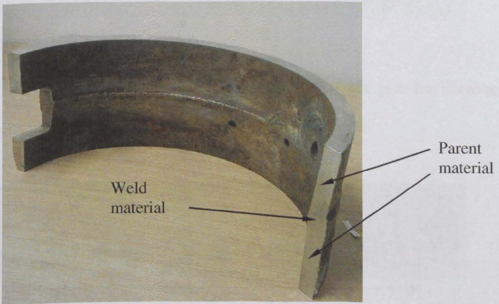
Figure 4.4 A photograph of the semi girth welded pipe.
