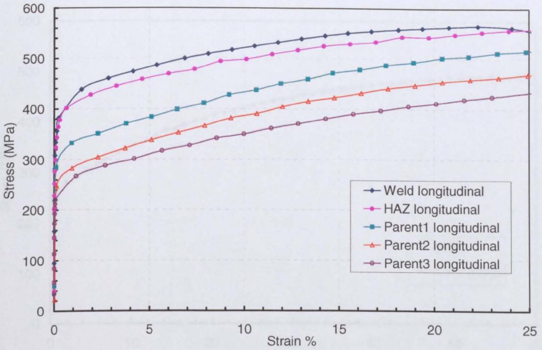
Figure 4.13 The DIC stress-strain curves of micro-specimens extracted from five different regions with the orientation normal to weld line (i.e. Weld, HAZ, parent1, parent2, and parent3)
