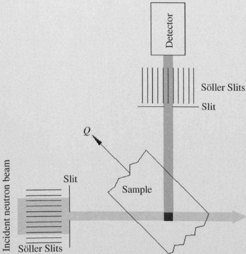
Figure 2.15 Schematic diagram of a neutron diffraction setup.
