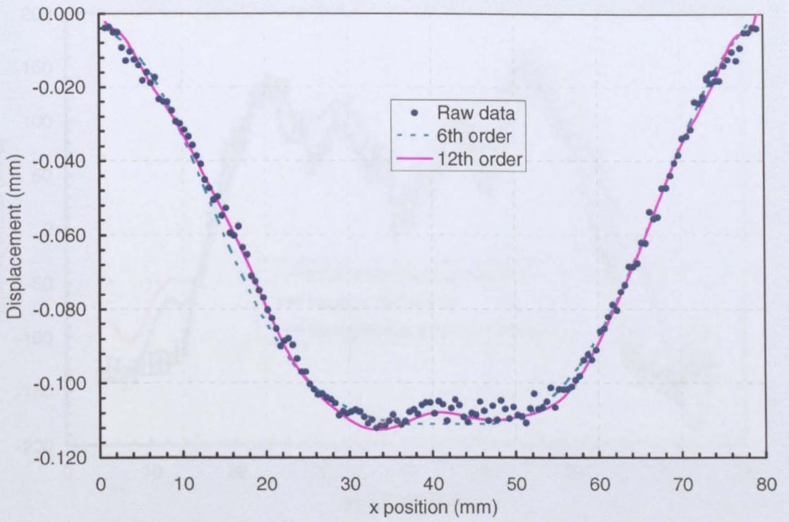
Figure 7.5 A comparison between fit data obtained by inverse solution for the order of 6<sup>th</sup> and for the order of 12<sup>th</sup> at  $y = 3.55$  mm on the  $\theta = 0^\circ$  surface.
