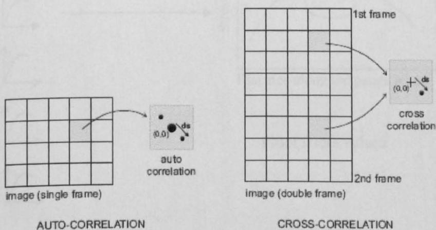
Figure 3.7 Schematic diagrams of auto and cross correlation [30].
