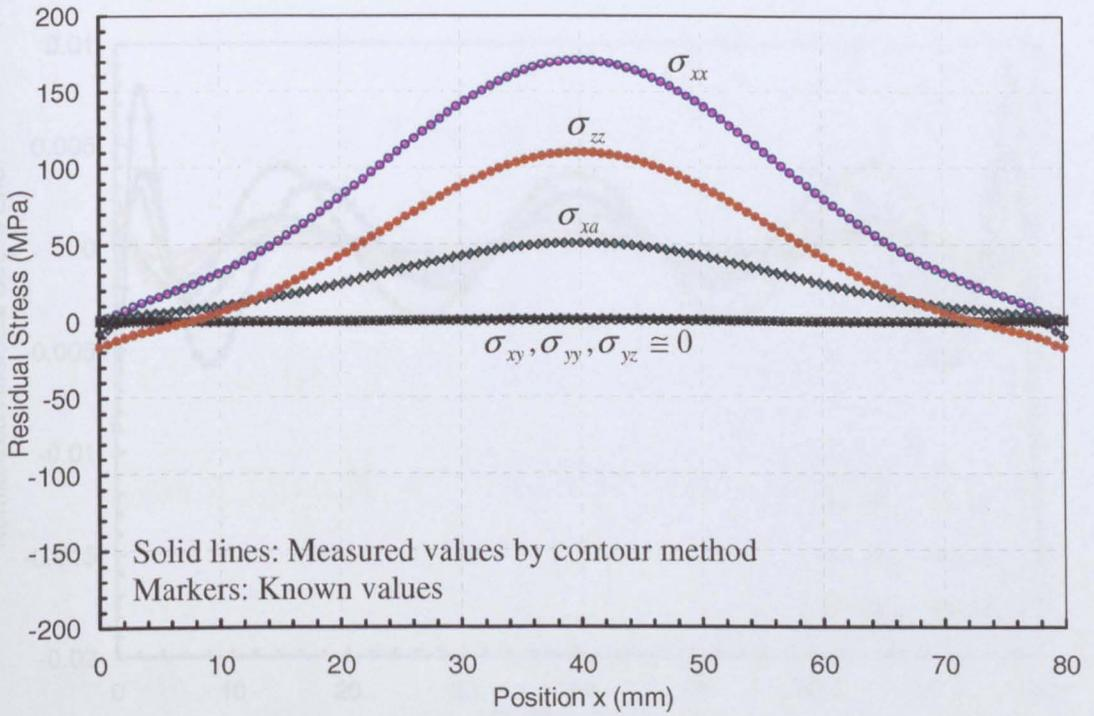
Figure 6.13 Comparison between known and measured residual stress for 3D numerical verification of the multi-axial method along the line  $y = 3.55$  mm
