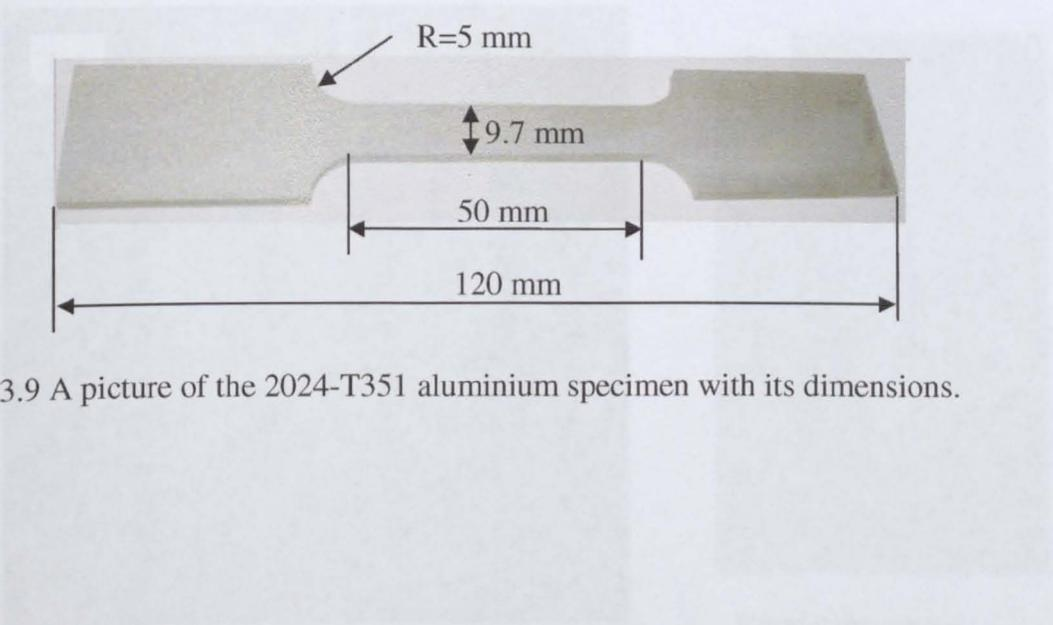
Figure 3.9 A picture of the 2024-T351 aluminium specimen with its dimensions.
