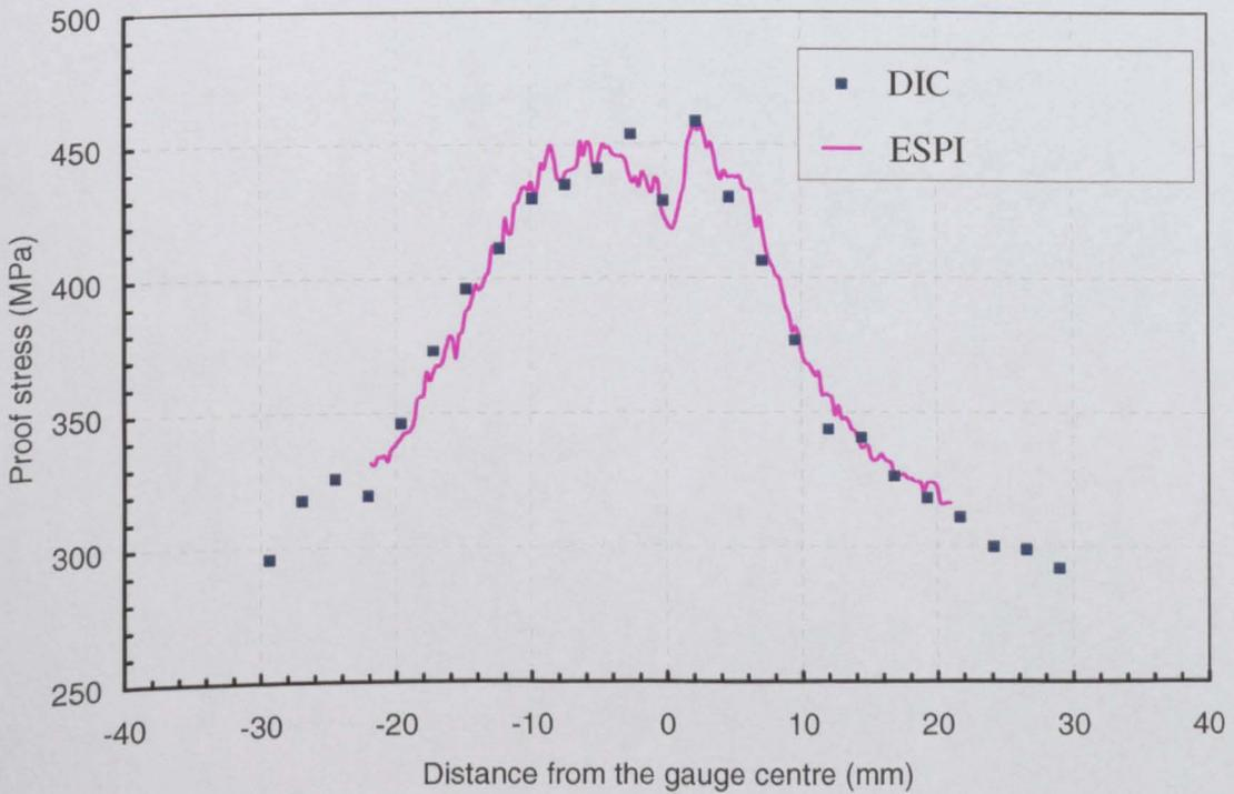
Figure 4.24 Variation of 0.5% proof stress along the length of the standard specimen
