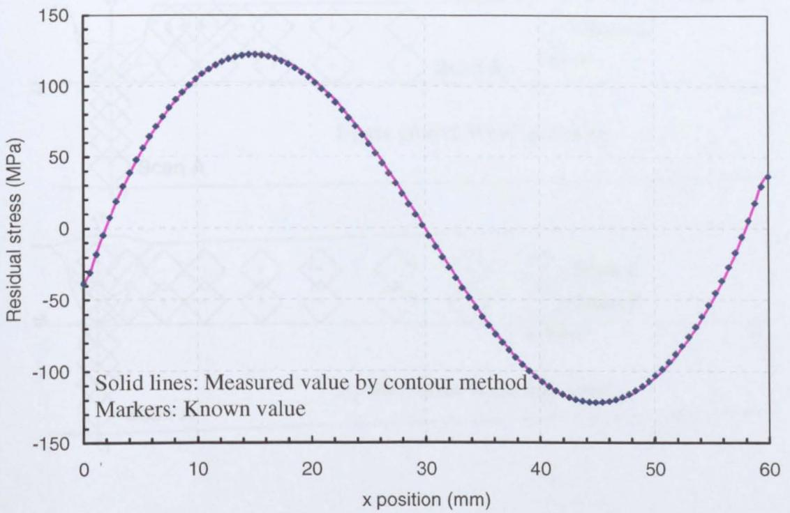
Figure 5.10 Comparison known and measured residual stress component normal to the cut surface for 3D numerical verification of contour method along the line  $y=7.5$  mm.
