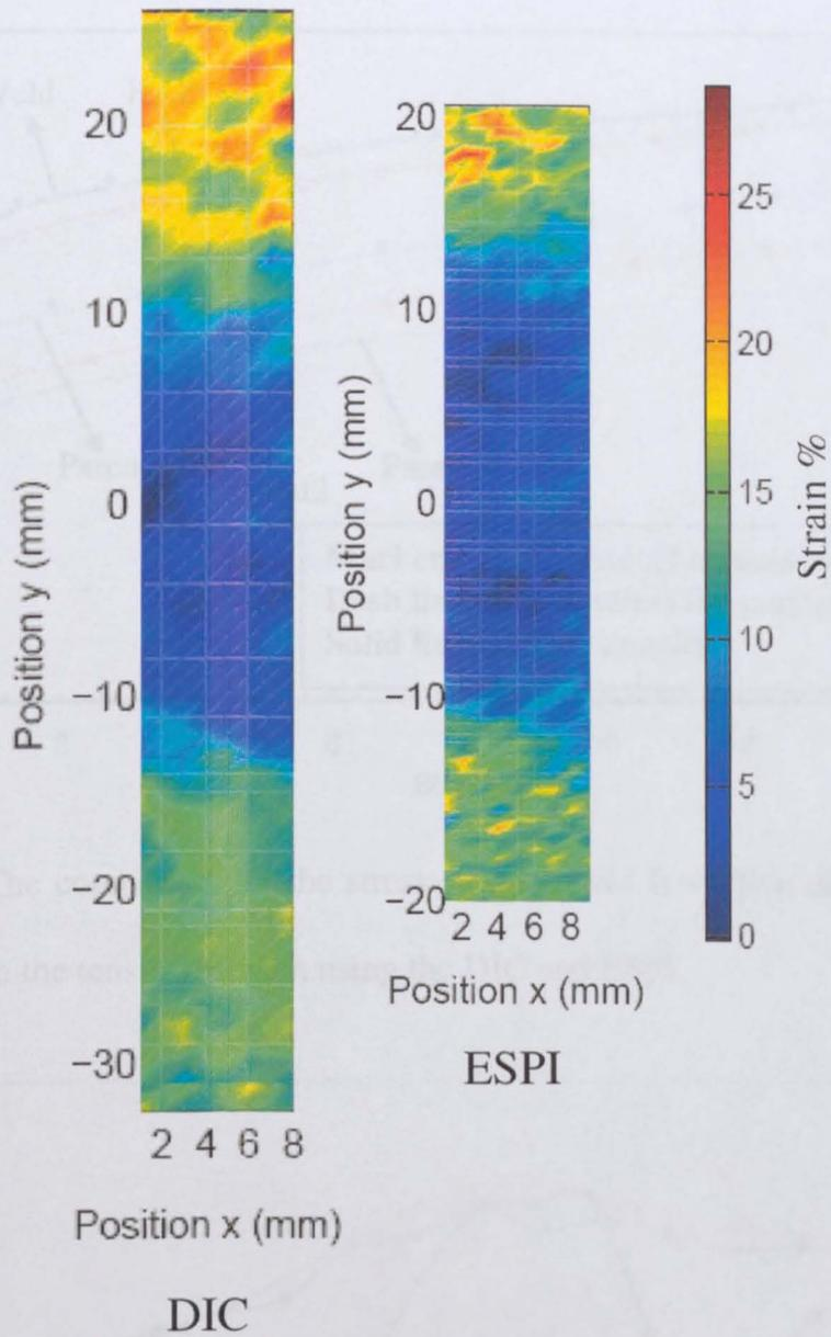
Figure 4.20 Longitudinal strain distributions in the gauge of the standard tensile specimen using DIC and ESPI techniques at an applied stress of 455 MPa.
