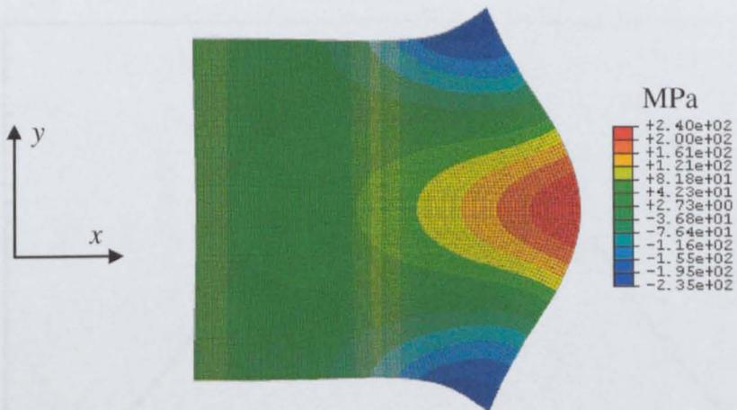
Figure 5.5 Map of the residual stress  $\sigma_{xx}$  for 2D numerical validation of the contour method. Magnification of deformation is 300.
