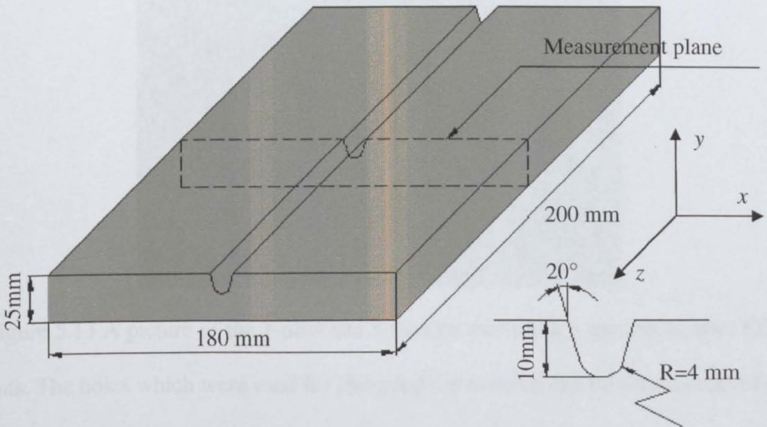
Figure 5.11 Schematic of the groove weld blank before welding and the geometry of the groove.
