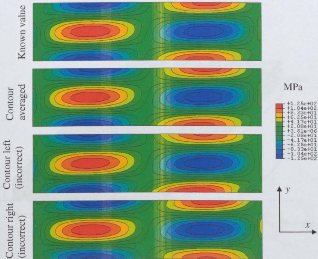
Figure 5.9 Known and calculated residual stress profiles.
