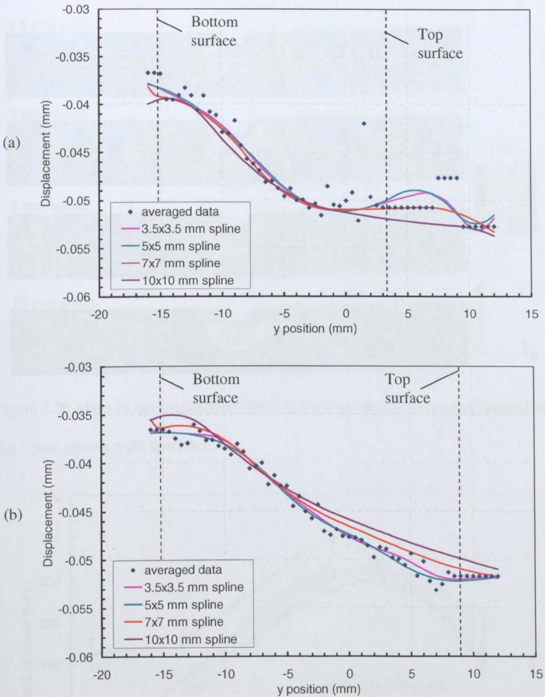
Figure 5.19 The comparison between the averaged data and four different spline knot spacings for the 1 pass groove weld specimen along the lines (a)  $x=0$  mm and (b)  $x=8$  mm (after removing the rows of data points on the top surfaces).
