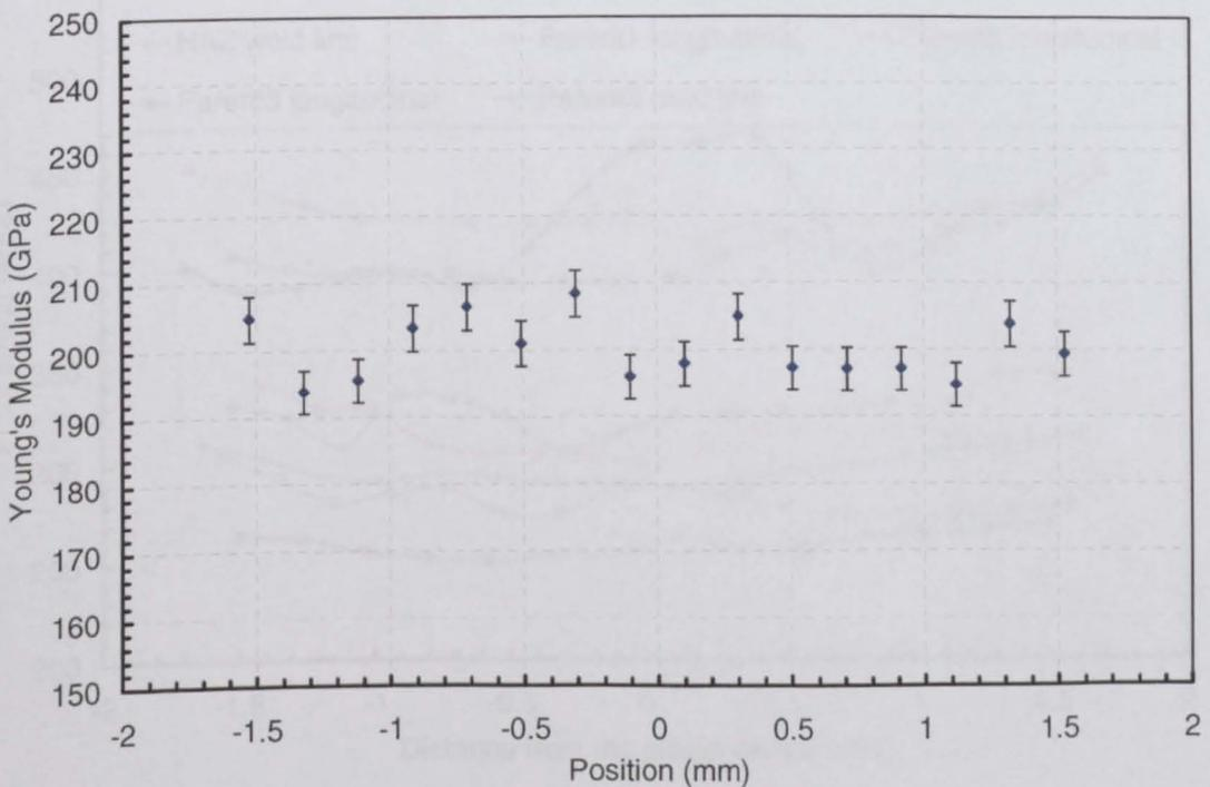
Figure 4.16 The variation of Modulus of Elasticity along the micro tensile test sample extracted from the HAZ region in the weld line direction.
