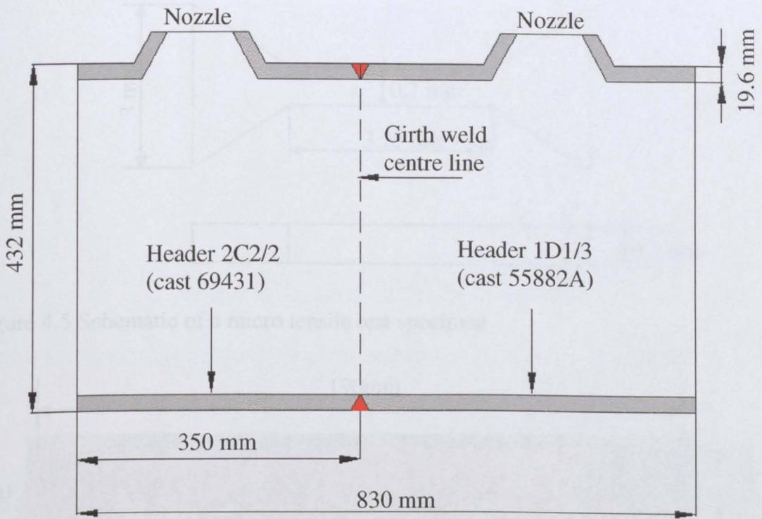
Figure 4.3 Schematic of the girth welded pipe
