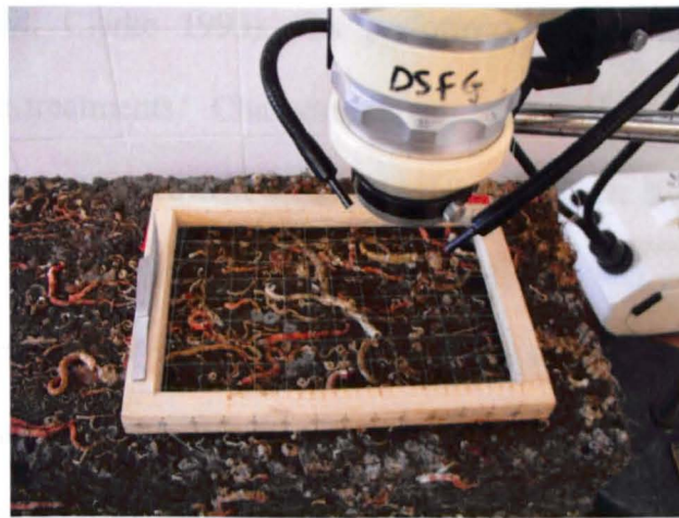
Figure 5.4. Analysis of epifaunal abundance of a reef block using a boom-mounted binocular microscope and a wooden grid with 100 counting squares.
