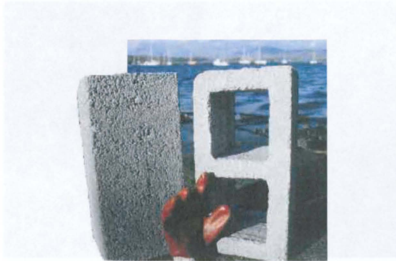
Figure 1.3. Simple (left) and complex (right) reef blocks made at Glensanda quarry for the Loch Linnhe artificial reef complex. Blocks are 42 x 21 x 21cm. Image used courtesy of Tom Wilding.
