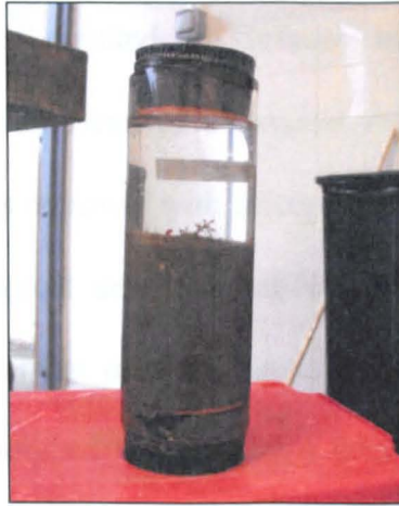
Figure 5.2 100mm diameter perspex sediment core with sediment sample prior to sieving.
