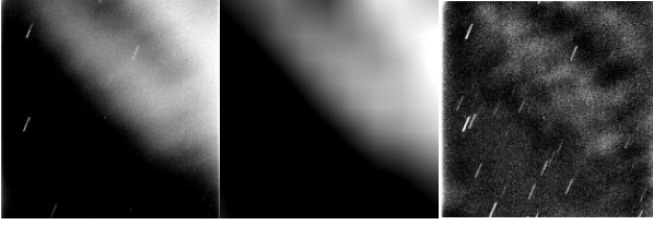
Figure 2: Sample frame obtained with a telescope in a non-sidereal tracking mode (left). Background estimated using the described method (centre). Original frame with the background subtracted (right).
