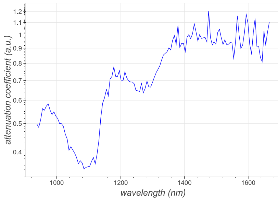
Figure 4.5: (a) Measured NIR transmission spectrum. (b) Absorption spectrum of blood extracted from time-dependent component of the NIR measurement. In contrast to the visible spectra, due to less absorption by skin and other surrounding
