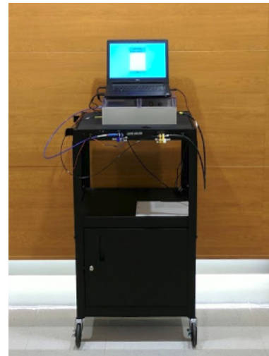
Figure 4.1: (a) Spectroscopy system setup diagram. The spectrometers, microcontroller and associated circuitry, and halogen lamp are all enclosed in a plastic container for protection and efficient disinfecting. (b) Spectroscopy system on portable cart for convenient transport between patients. The laptop computer rests on the plastic container, and the UPS is enclosed in the lower compartment of the cart.
