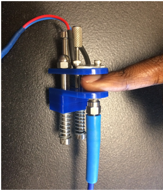
Figure 4.2: Clip design for (a) visible and (b) NIR spectral measurements. The visible design includes the LED light source on the clip itself while the halogen lamp, which acts as the NIR light source, is positioned on the cart, and the light is directed to the clip via liquid light guide.
