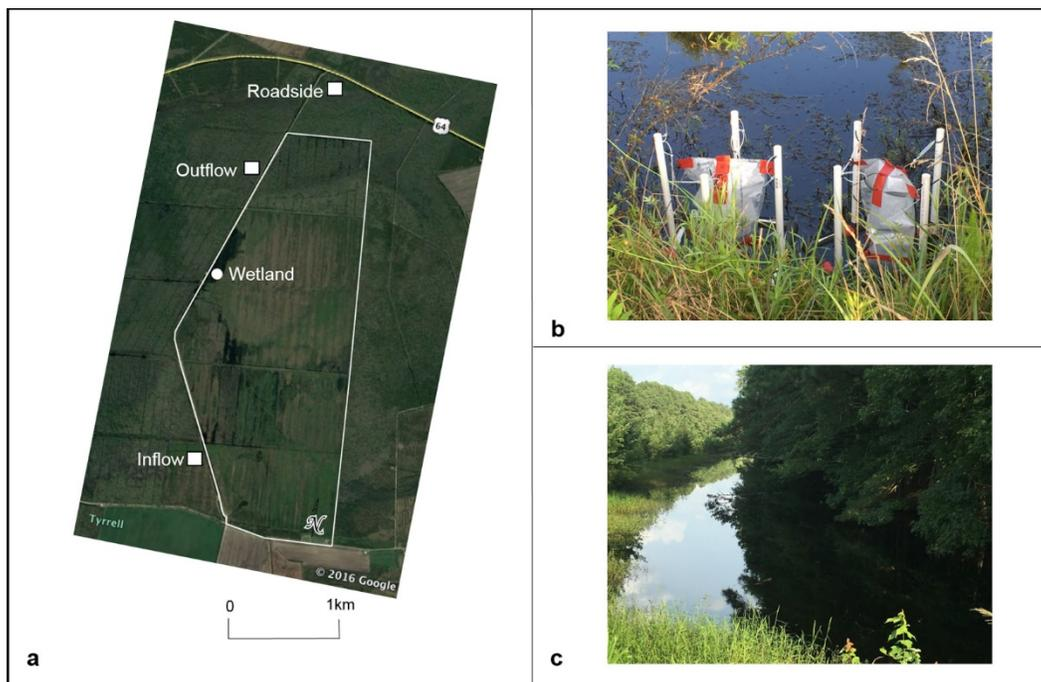
**Figure 2:** (a) Sample sites within the Timberlake Observatory for Wetland Restoration, including sites from this study (squares) and Wetland data from Carmichael et al. (2018) (circle) for comparison purposes; (b) deployed floating static flux chambers for the measurement of water-atmosphere greenhouse gas fluxes; (c) representative image of a wetland drainage canal. The image in panel (a) was created using Google Earth (copyright by DigitalGlobe).
