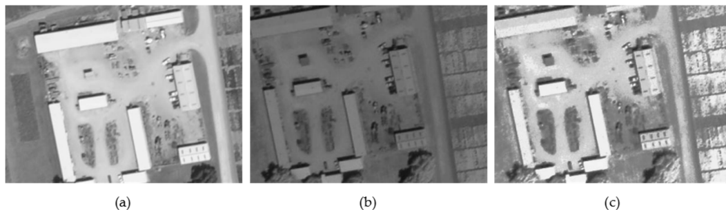
Figure 7. Images before and after specification: (a) RGB grayscale image; (b) initial NIR grayscale image; and (c) NIR grayscale image specified to RGB grayscale image.
