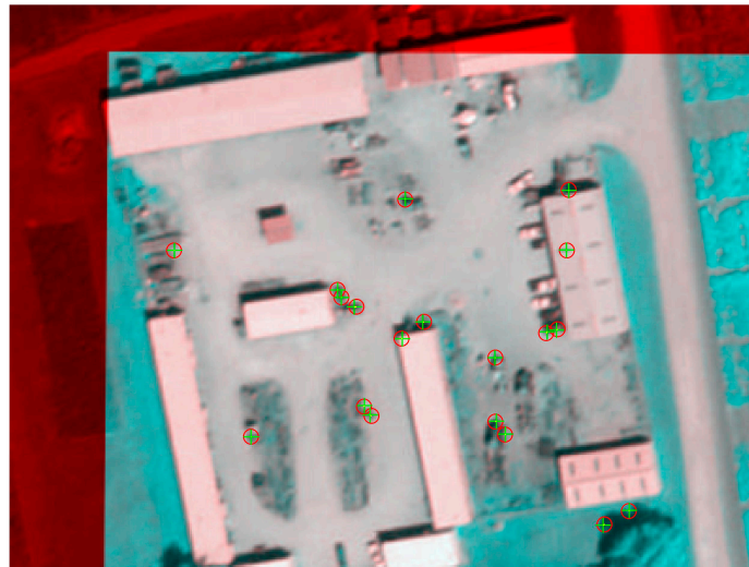
Figure 9. Overlap of the reference image in the bottom (NIR image) with the sensed image on the top (RGB image) with affine transformation, based on the FAST matched points. The red circles indicate the feature points on the NIR image and the green plus signs represent those on the RGB image. The red and green point pairs shown in this figure were the correct matching pairs, after elimination by m -estimator sample consensus (MSAC).
