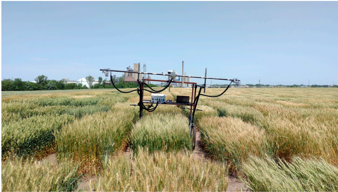
Figure 6. The slanting issue of the phenocart.
