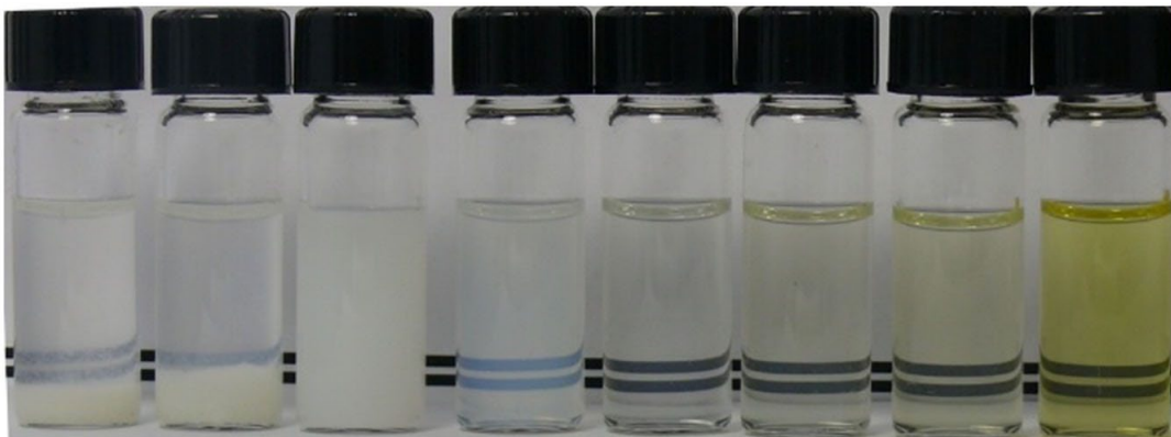
Fig. 2. Appearance of the emulsion containing 38.5 mg/mL eugenol after 20-fold dilution in PBS adjusted to pH 2.5, 3.0, 4.0, 5.0, 6.0, 7.0, 8.0 and 9.0 (from left to right)
