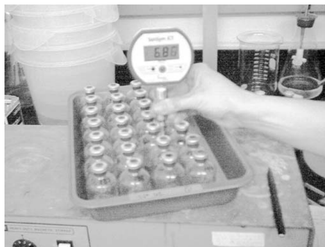
Fig. 1 Digital gauge used for measurement of gas pressure in sealed vials
