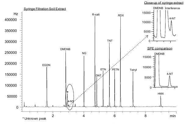
**Fig. 5.** Chromatogram of fortified potting soil (2 µg/g) extracted with acetone, processed by syringe filtration, and analyzed by GC/ECD. Close-ups of the syringe and NEXUS SPE extracts around the elution time of 4-NT are given to highlight the differences.
