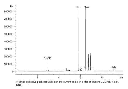
Fig. 3. GC/ECD chromatogram of Matrix 23, a sandy loam from a demolition range, following extraction with acetone and cleanup using the validated NEXUS SPE method. The peaks for TNT and RDX exceed the scale presented.
