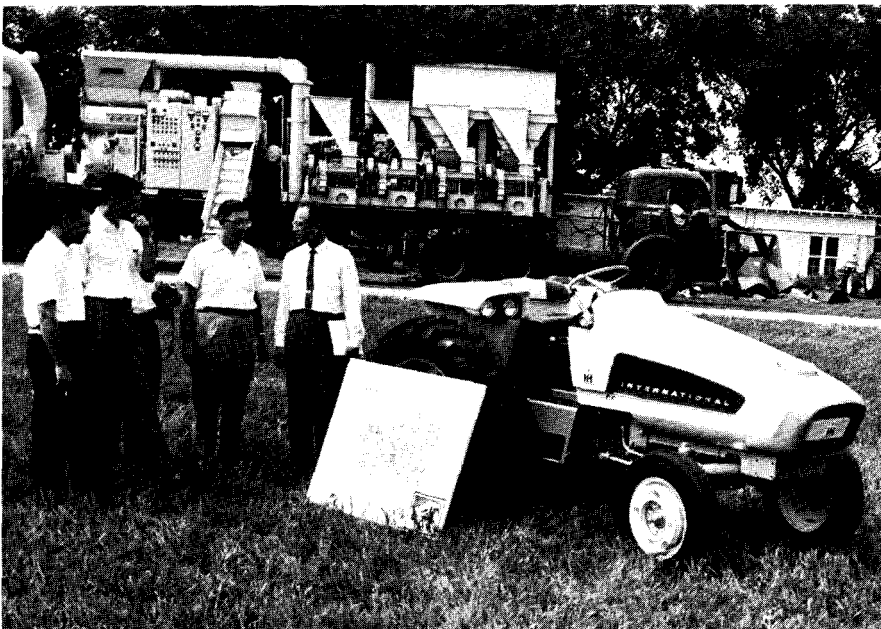
International Harvester displayed this new concept in engineering several years ago. This tractor paired a gas turbine with a hydrostatic transmission. The machine in the background is a pelletizer.
