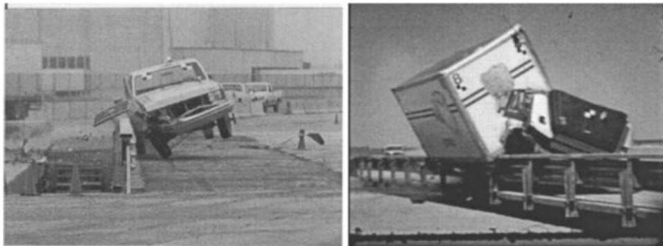
Fig. 2. Crash testing of FPL system
