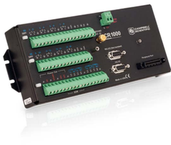
Figure 6. Datalogger (CR 1000 - Courtesy Campbell Scientific).
