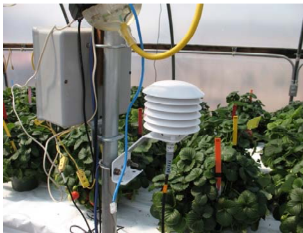
Figure 9. CS215 (SDI-12) Temperature and Humidity Sensor with Radiation shield,
