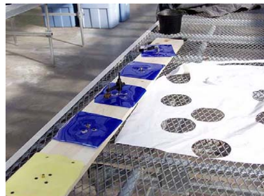
Figure 4. A pot cutter board system for alignment and placement of holes into plastic reflective mulch film for 6-inch pots of strawberries to access Cap Mat irrigation system. (Courtesy of Mr. Gary Deberg, Biological System Engineering Technician).
