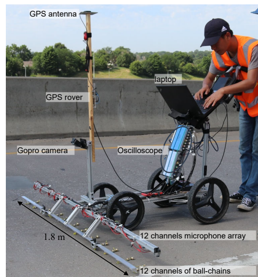
Figure 1. 12-channel acoustic scanning cart.
