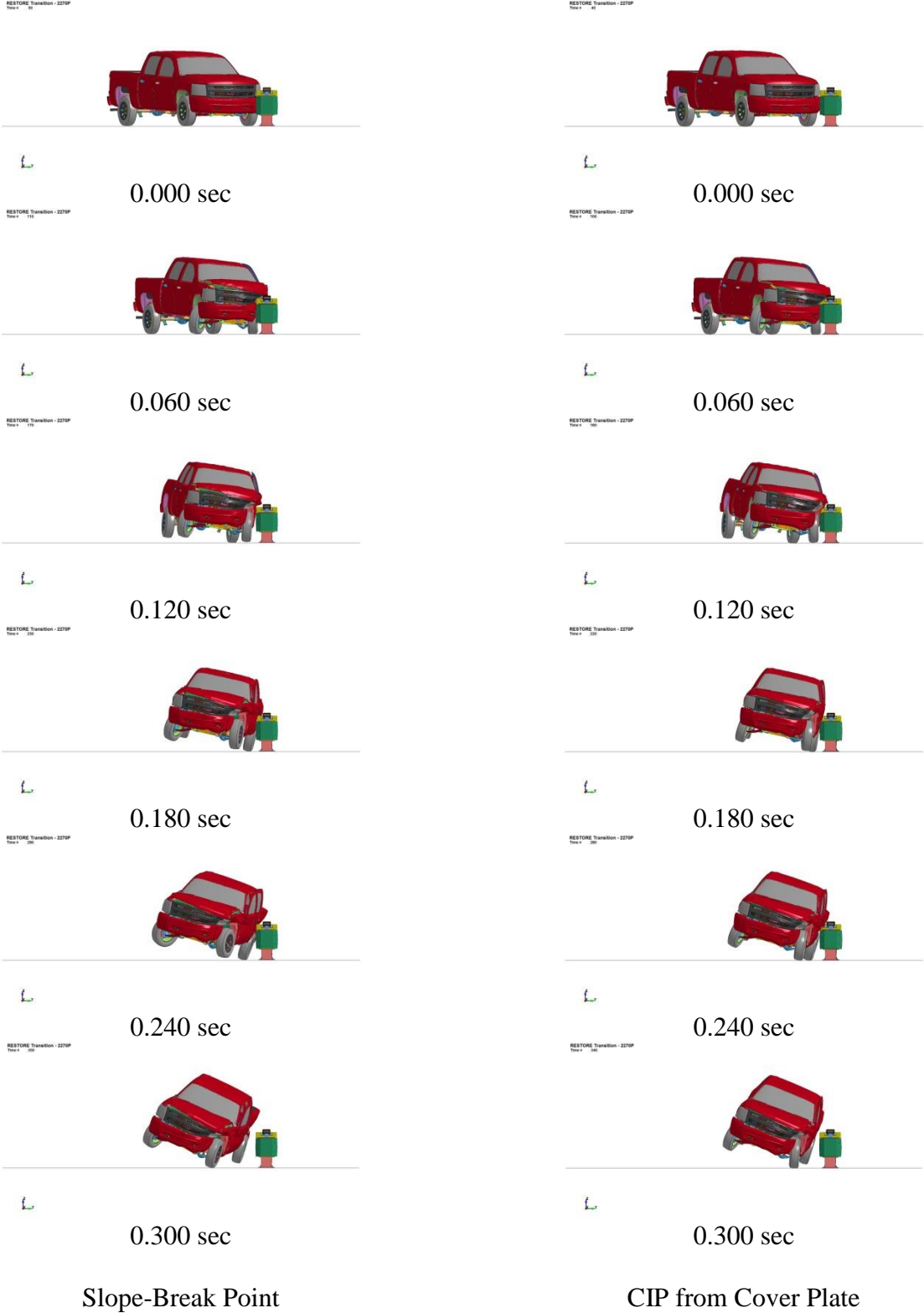
Figure 221. RESTORE Barrier Transition, 2270P Silverado Simulation Comparison, Reverse-Direction Locations, Downstream View
