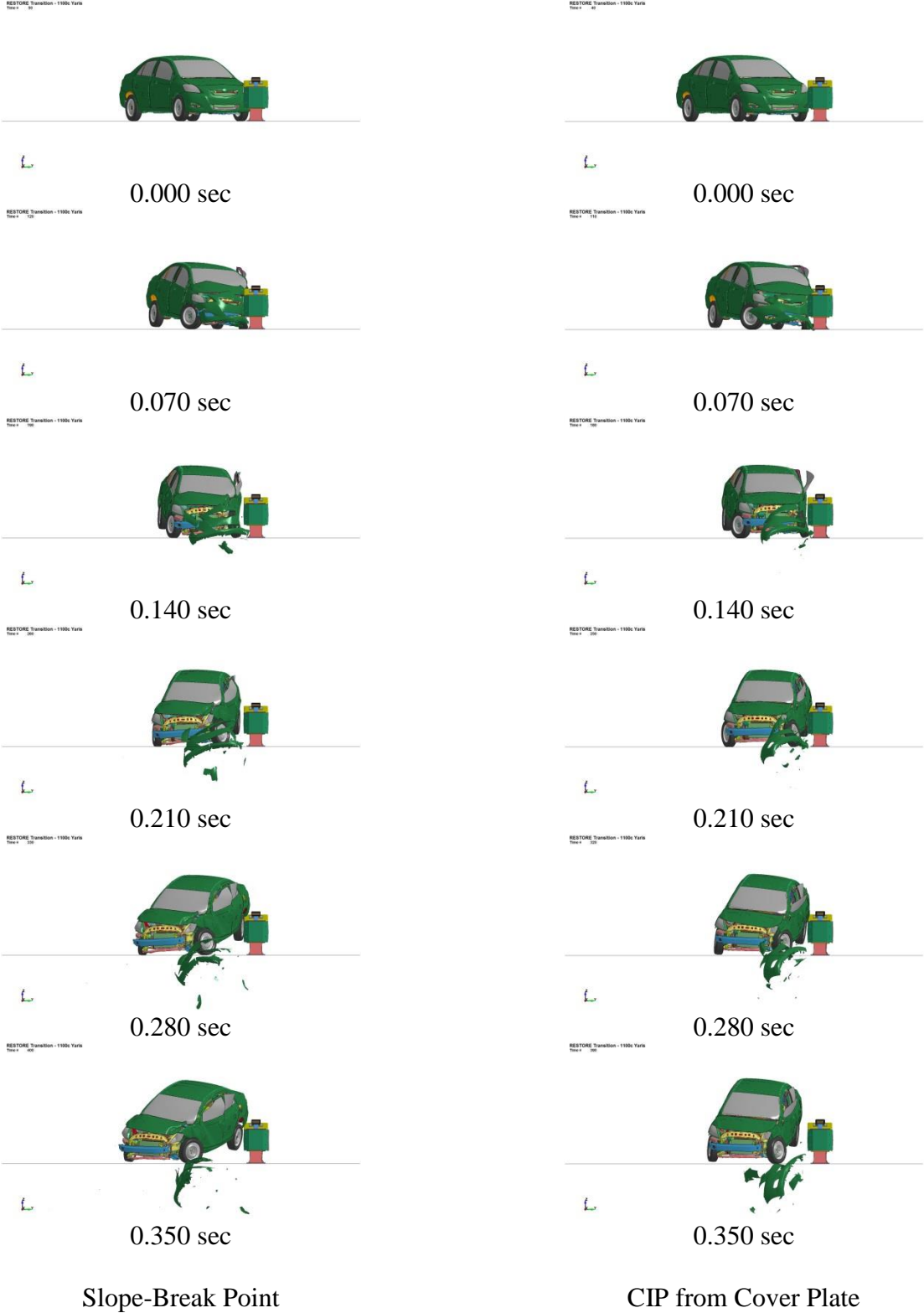
Figure 182. RESTORE Barrier Transition, 1100C Yaris Simulation Comparison, Reverse-Direction Locations, Downstream View
