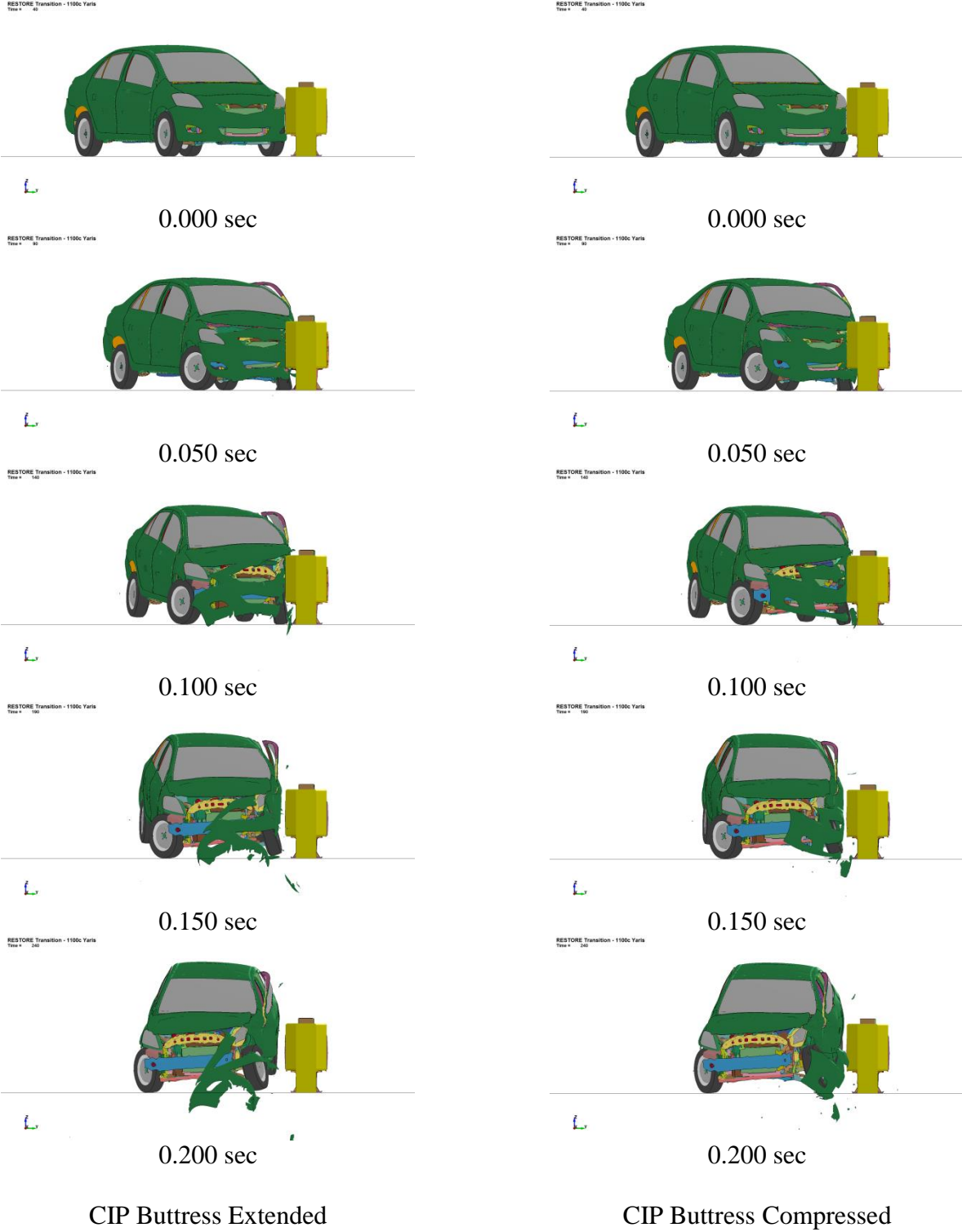
Figure 138. RESTORE Barrier Transition, 1100C Yaris Simulation Comparison, CIP Locations, Downstream View
