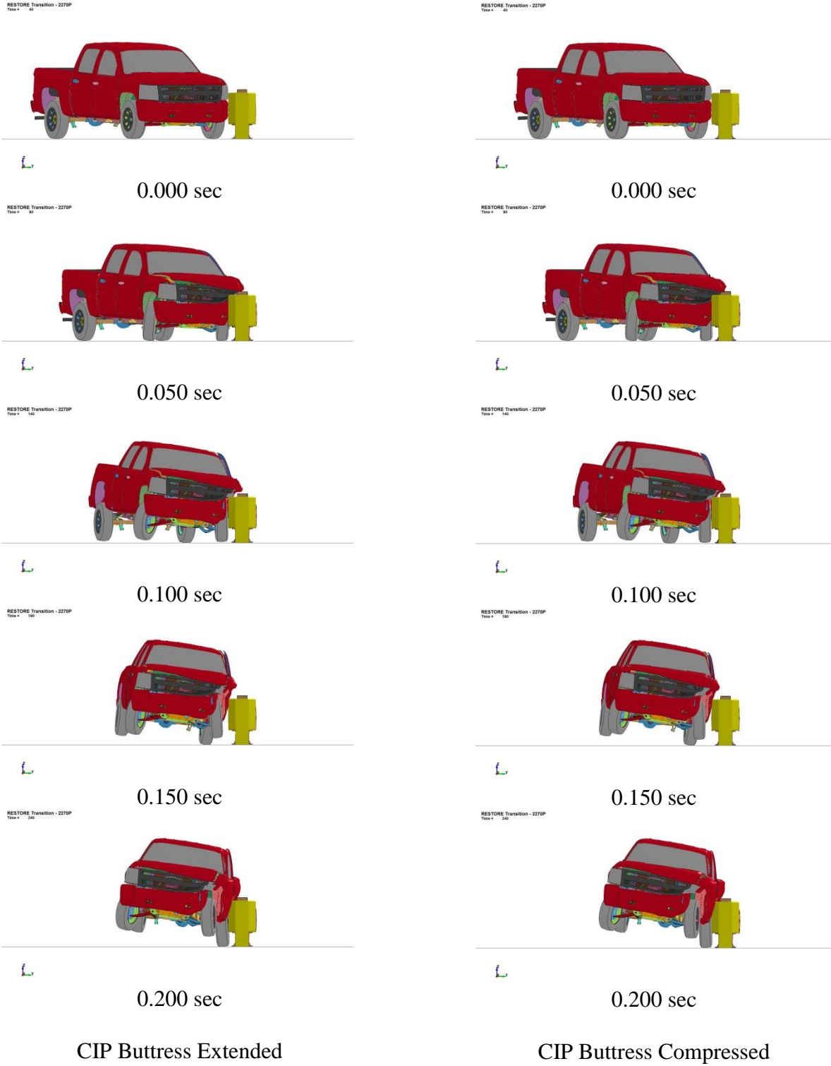
Figure 201. RESTORE Barrier Transition, 2270P Silverado Simulation Comparison, CIP Locations, Downstream View
