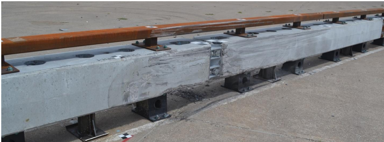
Figure 40. RESTORE Barrier Damage, Test No. SFH-1 [20-21]
