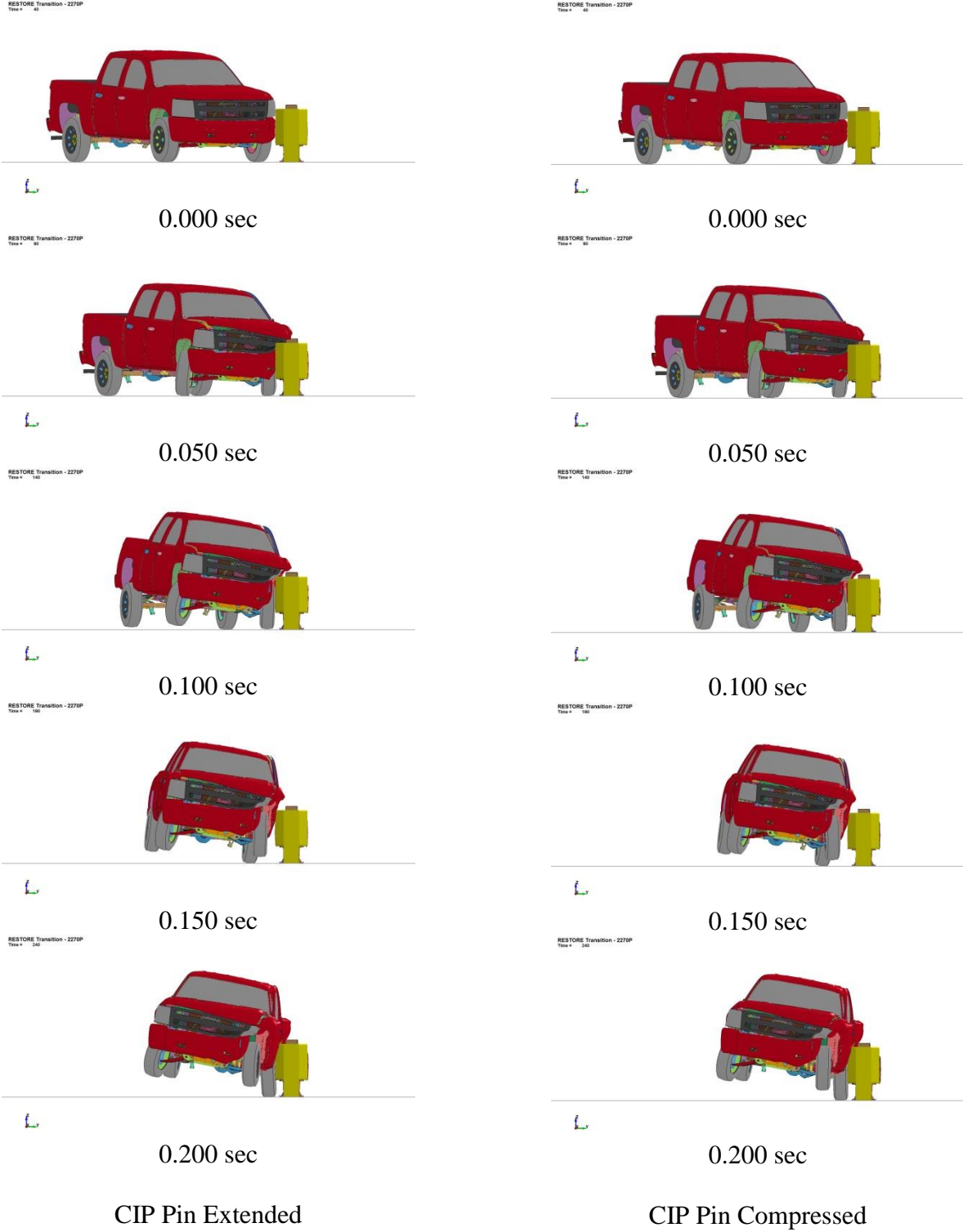
Figure 202. RESTORE Barrier Transition, 2270P Silverado Simulation Comparison, CIP Locations, Downstream View
