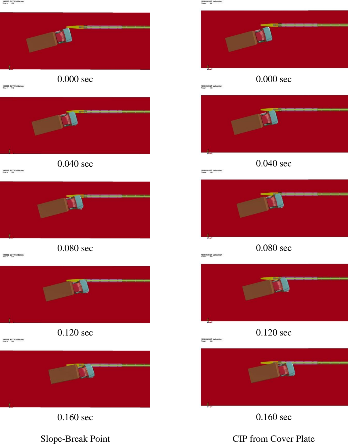
Figure 255. RESTORE Barrier Transition, 10000S F800 Simulation Comparison, Reverse-Direction Locations, Overhead View
