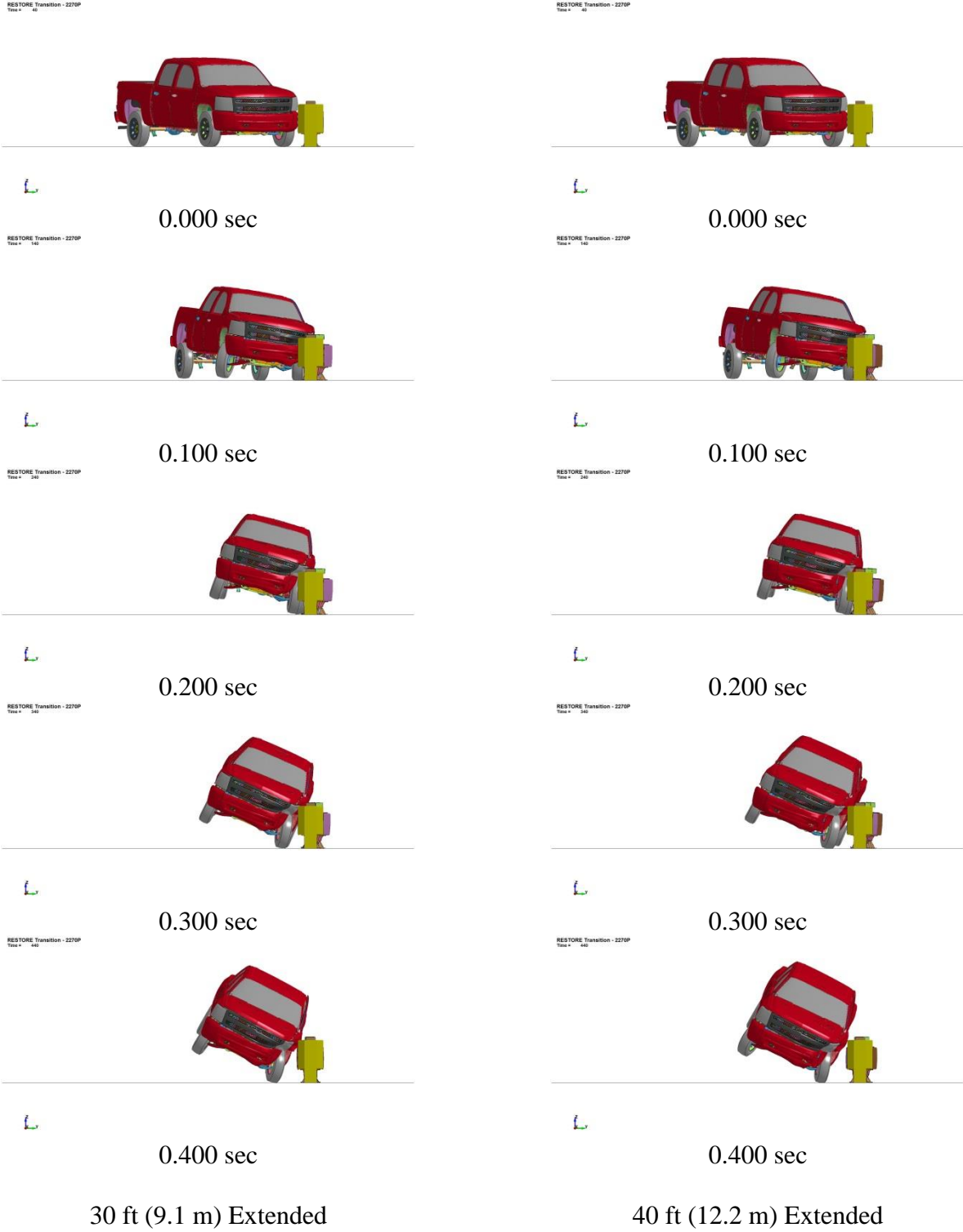
Figure 212. RESTORE Barrier Transition, 2270P Silverado Simulation Comparison, Upstream Impact Locations, Downstream View
