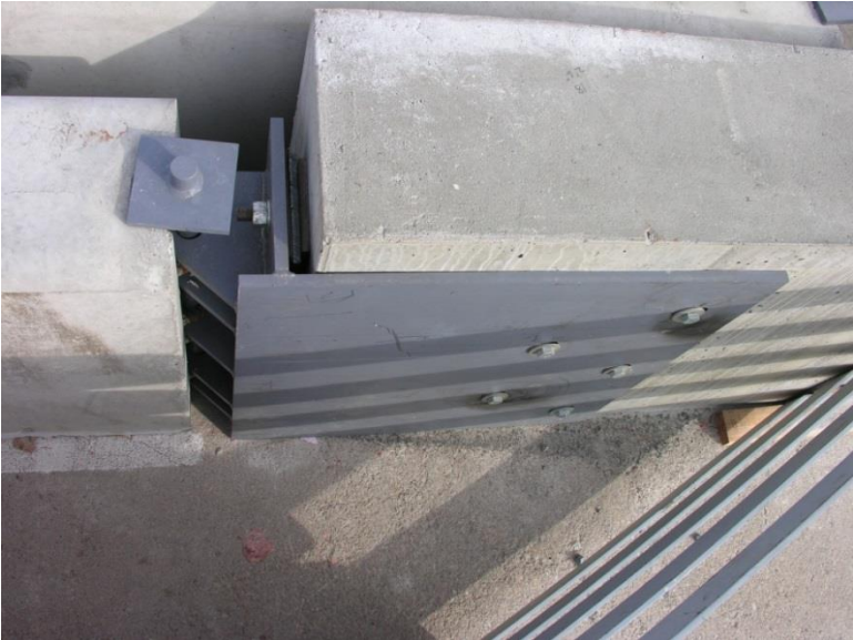
Figure 16. Pre-Test Photographs of SAFER on PCB Installed Across Opening, Test No. SPCB-1 [39-40]
