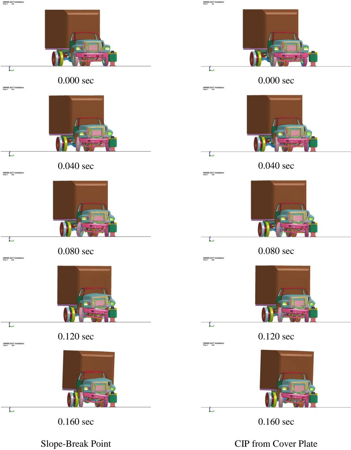
Figure 254. RESTORE Barrier Transition, 10000S F800 Simulation Comparison, Reverse-Direction Locations, Downstream View
