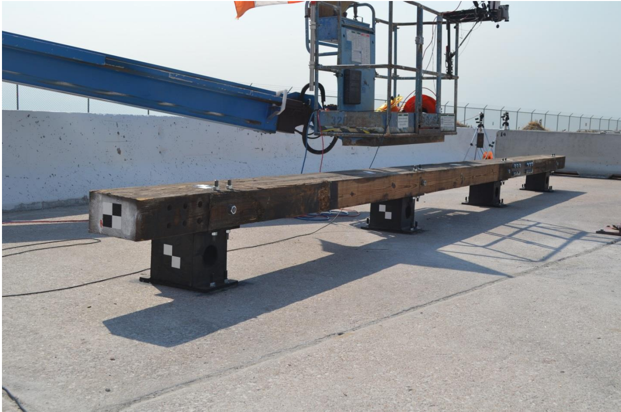
Figure 37. Bogie Test Setup for Beam and Shear Fenders, Test No. SFHT-1 [18]
