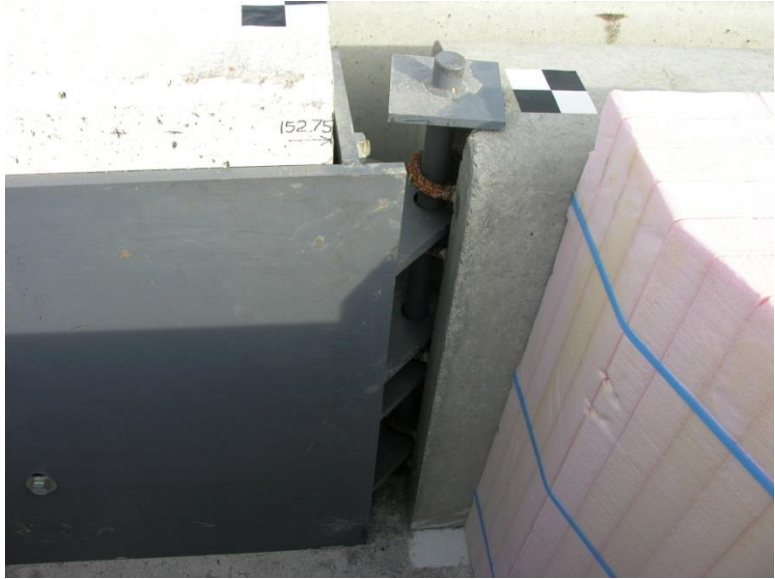
Figure 17. Pre-Test Photographs of SAFER on PCB Installed Across Opening, Test No. SPCB-1 [39-40]
