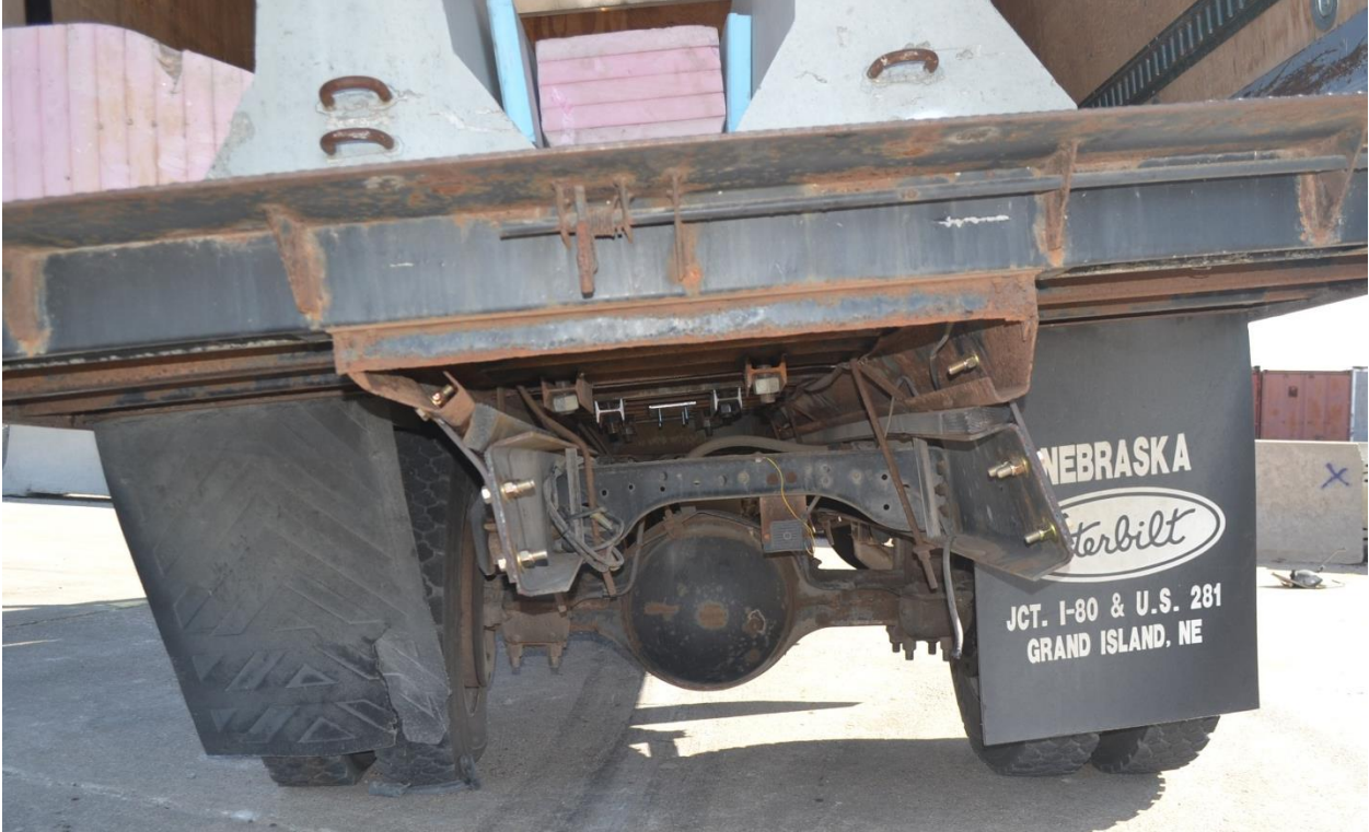
a. Full-Scale Test Box Attachment Damage
