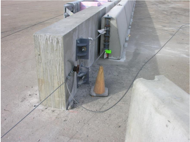
Figure 16. Pre-Test Photographs of SAFER on PCB Installed Across Opening, Test No. SPCB-1 [39-40]
