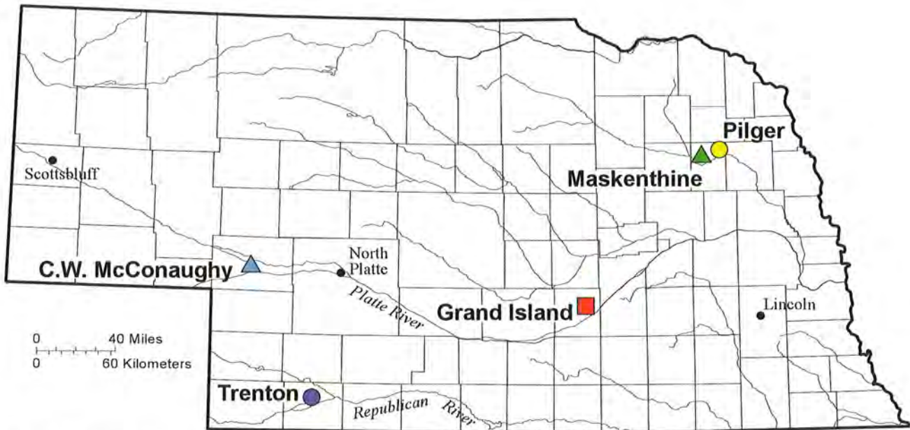
Figure 1. Location of grout study sites. Sites shown with a circle used bentonite slurry, bentonite chip and cement grout products; site shown with a square used bentonite slurry, bentonite chip, cement and bentonite thermal grout products; sites shown with a triangle used only bentonite thermal grout products.
