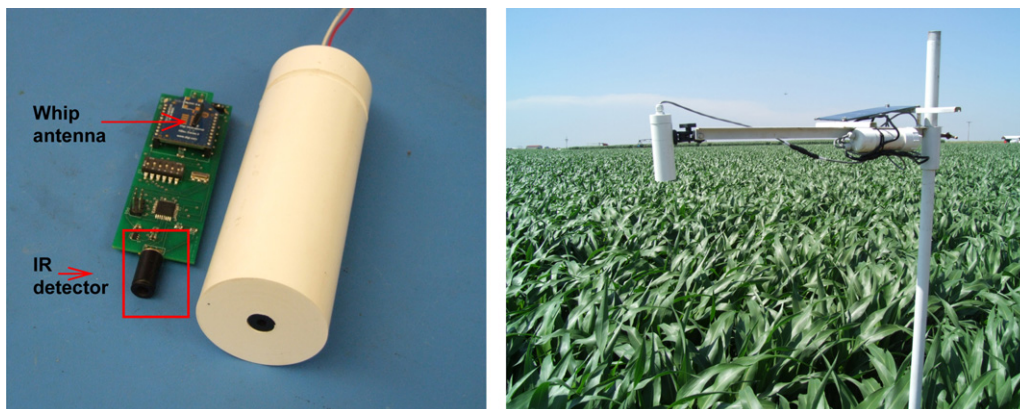
Fig. 3. Wireless infrared sensor module consisting of the collimated infrared detector (inside red rectangle), RF module and interfacing circuit on the left; and sensor inside of the white PVC housing on the right.
