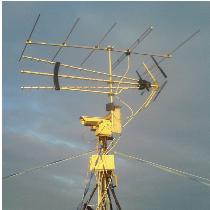
(a) Reference channel, FM radio antenna; TRIAX 5 element [127] (upper antenna), DVB-T antenna; Teledesic DAT75 Digital Tv Aerial [128] (lower antenna).
