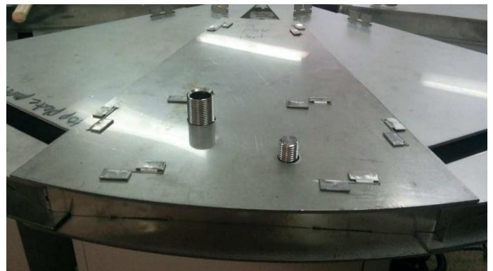
FIGURE 9: TABS BENT TO FASTEN THE MIXING ELEMENT'S TOP-AND BOTTOM-PANELS TO THE CHANNEL WALL-COMPONENTS.
