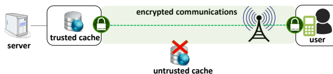
Fig. 1: End-to-end encryption precludes untrusted caches, and limits caching to trusted entities. This paper proposes a new security protocol to enable caching encrypted content and encourage the operation of untrusted caches.
