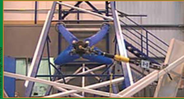
Fig. 9: Testing early version with hydraulic systems replicating broken wire conditions.
