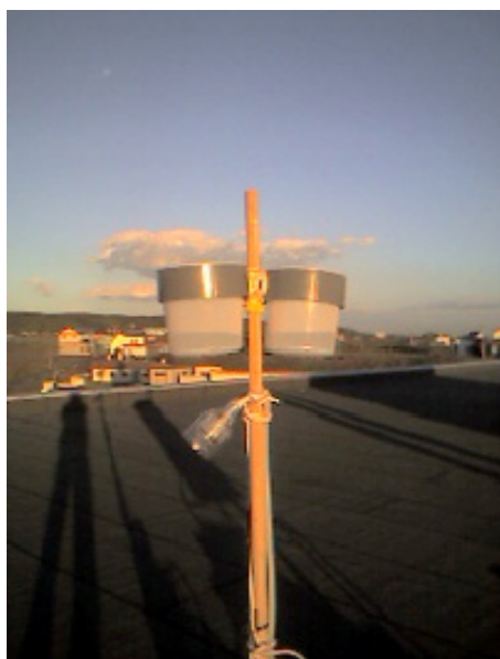
Figure 2 Total deposition sampler at Kushiro. Two Buckets filled by water were set in 1.8m heights on the roof of Hokkaido National Fisheries Research Institute, Fisheries Research Agency in Kushiro.
