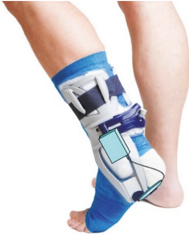
Figure 6: View of a possible mounting of the system on an orthosis. The piezo buzzer and sensors are placed at the bottom, the microcontroller is mounted on the side (Source: Colourbox, modified).
